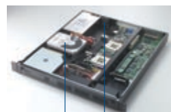
One internal 3.5" disk drive One rear 10-CFM cooling fan
