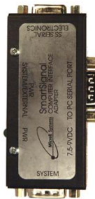
RS 232 Interface Adapter The adapter provides connections to a PC, the encoder system and the controller.
