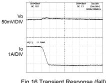
Fig.16 Transient Response (fall) 47u MLCC+30m  $\Omega$
