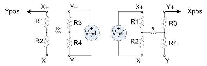
Figure 14. Ordinate (Y) and abscissa (X) coordinates measurement setup
