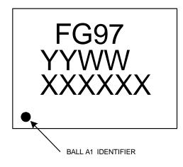
Figure 2. SX8652 WLCSP Top View, Solder Bumps on Bottom Side
