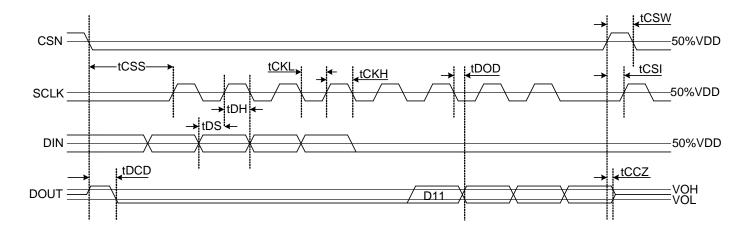
Figure 4. SPI Timing Waveform
