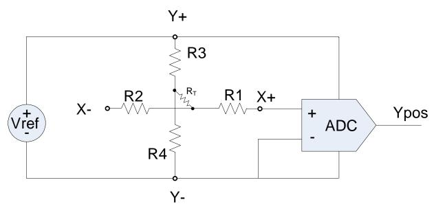
Figure 13. Touch Screen Operation ordinate measurement (Y)
