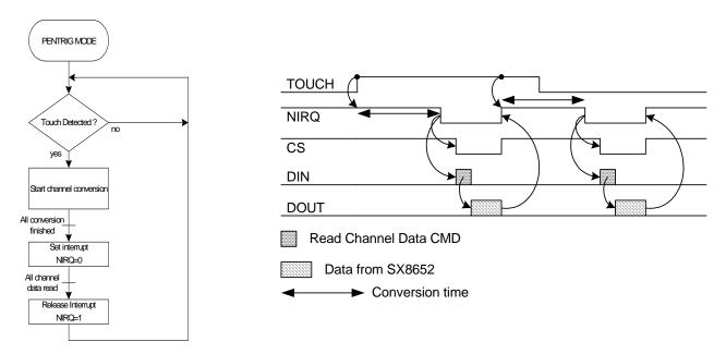
Figure 25. PENTRIG Mode Flowchart and SPI working in PENTRIG mode
