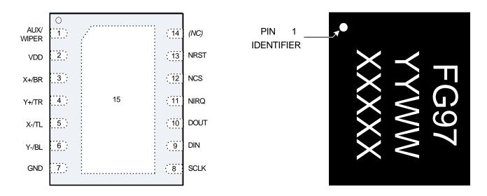
Figure 1. SX8652 DFN Top View, Pad on Bottom Side
