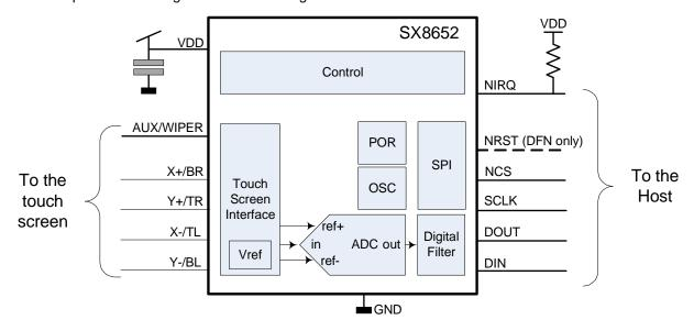
Figure 3. Simplified block diagram of the SX8652
