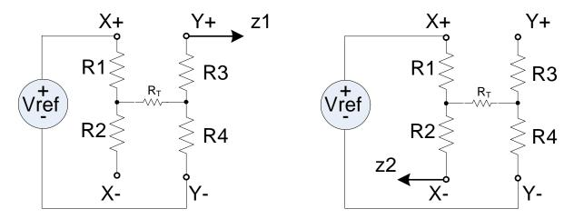
Figure 15. z1 and z2 pressure measurement setup
