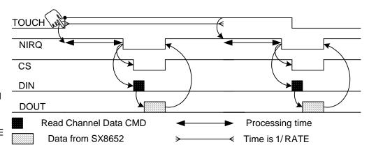
Figure 23. SPI working in AUTO mode
