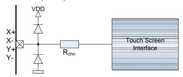
Figure 7. Simplified diagram of touchscreen pins
