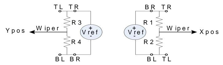
Figure 18. Ordinate (Y) and abscissa (X) coordinates measurement setup
