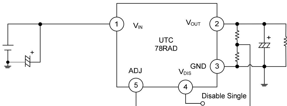
\*  $C_L$  is required if regulator is located an appreciable distance from power supply filter. [ $C_L > 0.33\mu F$  (Electrolytic)]
