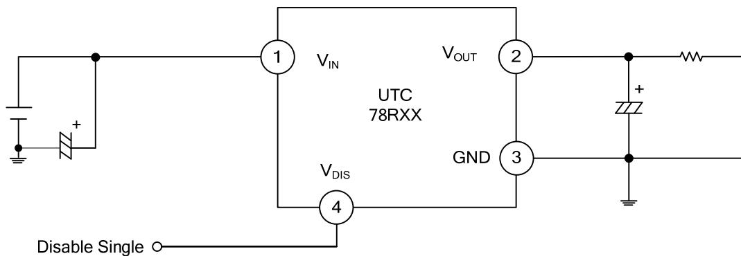
\*  $C_L$  is required if regulator is located an appreciable distance from power supply filter. [ $C_L > 0.33\mu F$  (Electrolytic)]
