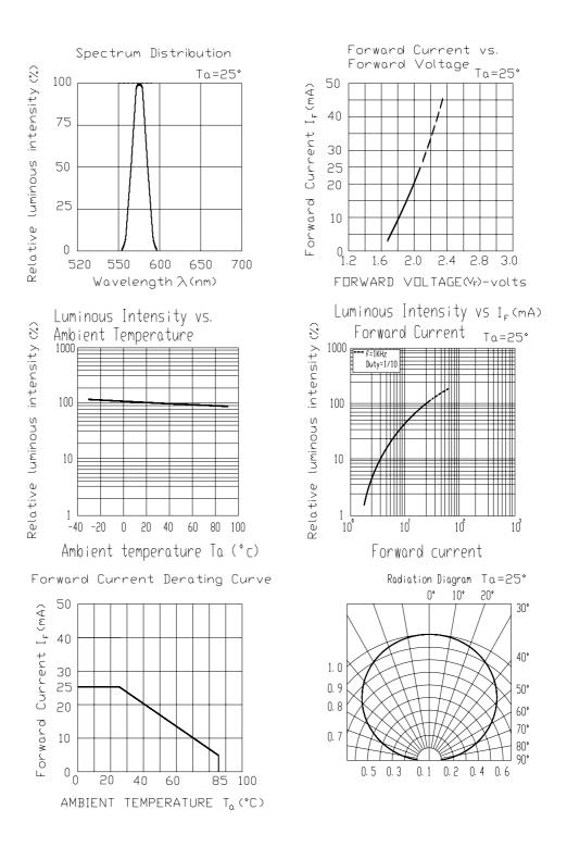
Everlight Electronics Co., Ltd. Device No. : DSE-942-043 http://www.everlight.com Prepared date: 22-Sep-2005 Rev. 2 Page: 4 of 6 Prepared by: Ray Yuan
