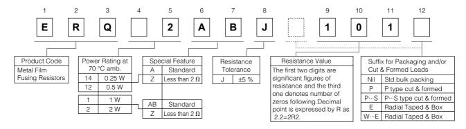
The above example shows a standard Metal Film Fusing Resistors, 2 W power rating, resistance value of 100  $\Omega$ , tolerance of  $\pm 5$  %, and package of standard bulk packing
