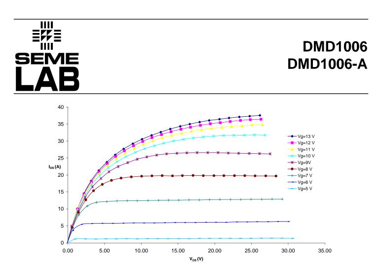
Figure 4 – Typical IV Characteristics.
