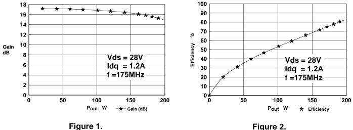
Figure 1. Gain vs.Output Power
