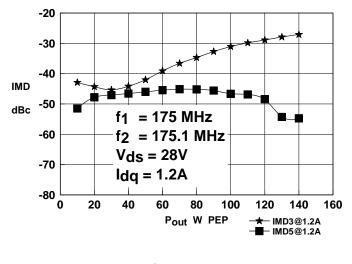
Figure 3. IMD vs Output Power
