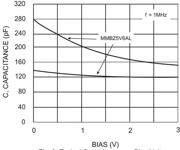
Fig. 3 Typical Capacitance vs. Bias Voltage
