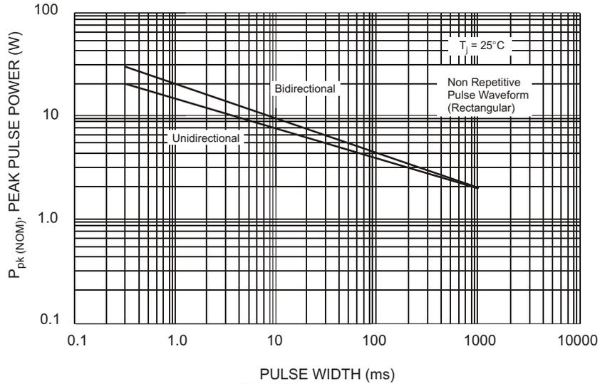
Fig. 7 Pulse Rating Curve,
