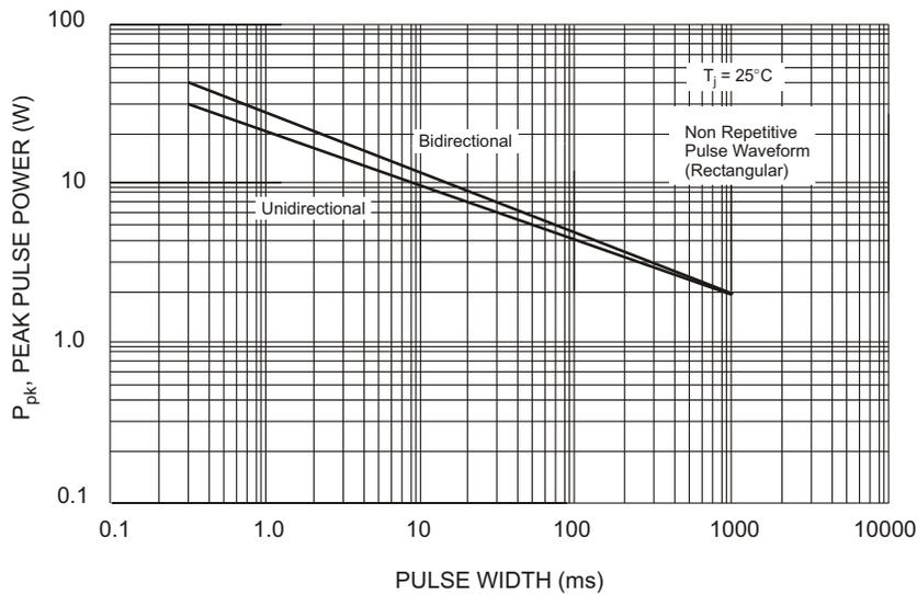
Fig. 6 Pulse Rating Curve,
