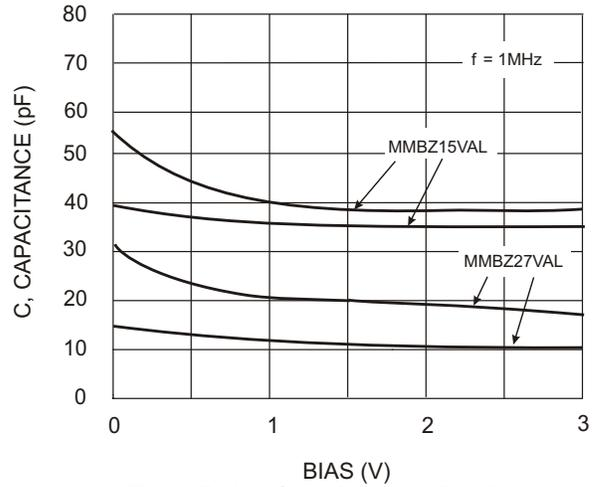
Fig. 4 Typical Capacitance vs. Bias Voltage
