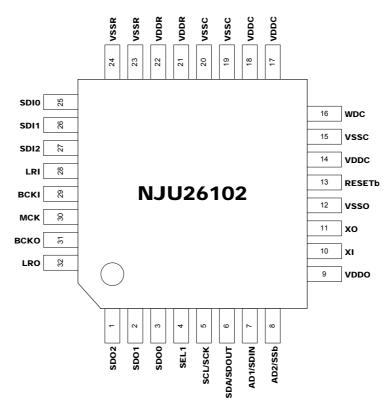
Fig. 3 NJU26102 Pin Configuration
