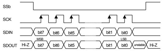
Fig. 4 4-Wire Serial Interface Timing
