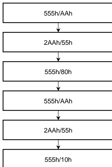
Auto Chip Erase Command Sequence (address/data)
