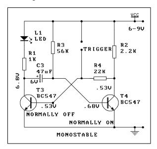
on, T3 turns off and so does the LED. The state is then stable again.
