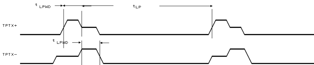
Transmitted Link Integrity Pulse Timing
