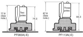
Note: PF083A(-E) and PF113A(-E) allow either track or screw mounting.
