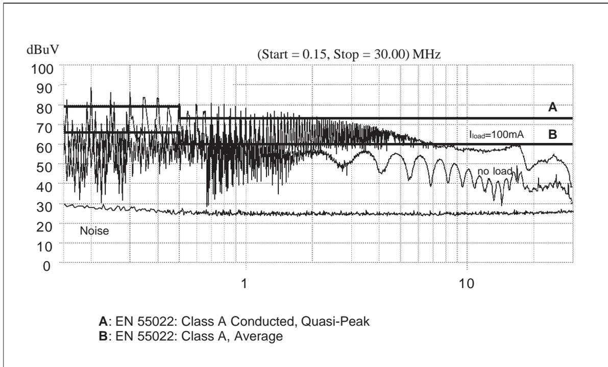
**Figure 19:** Buck converter with  $V_{out} = 16V$ : EMI behavior with EMI input filter
