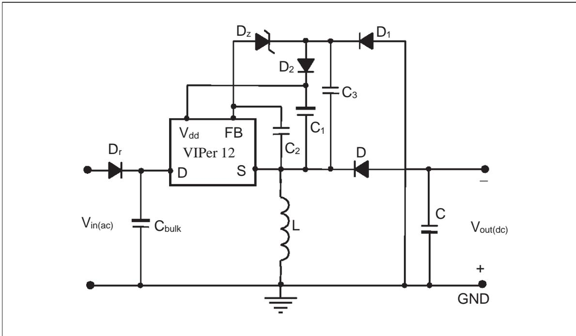
**Figure 26:** Buck-boost converter with  $-8V < V_{out} < 0$
