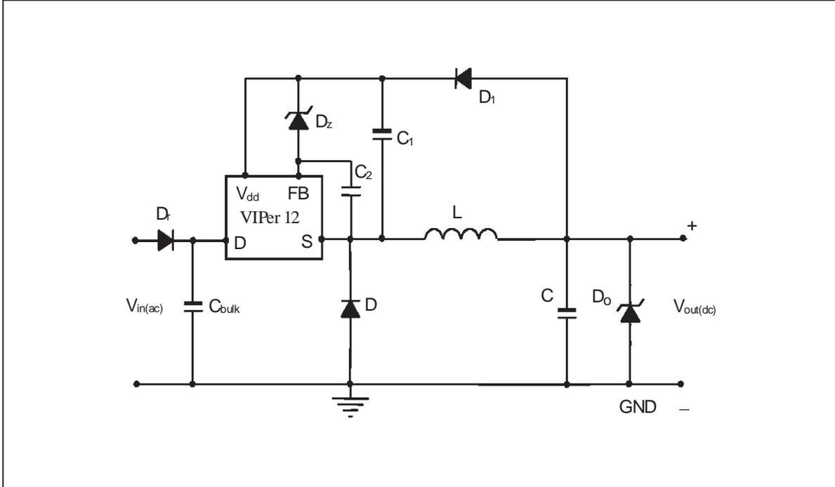
Figure 5: Buck converter with  $V_{out} < 15V$
