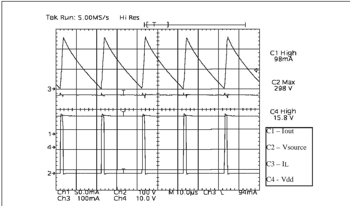
Figure 12: Buck converter with  $V_{out}=16V$ : open load condition
