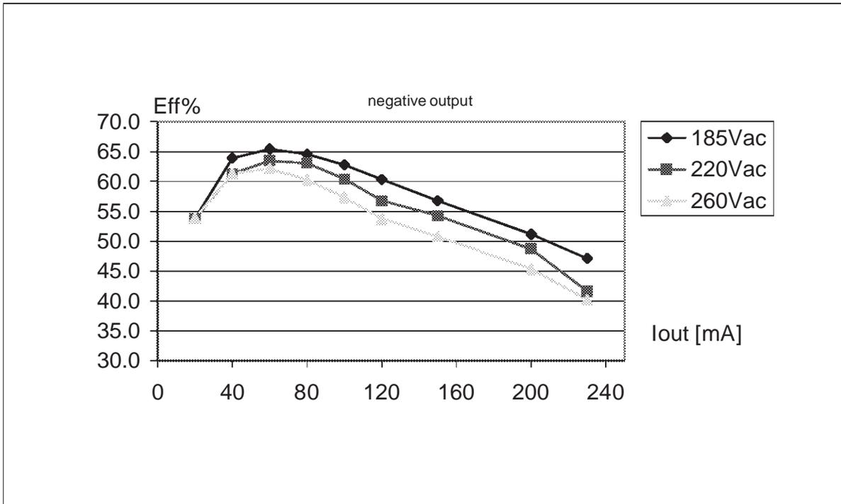
Figure 30: Buck-boost converter with  $V_{out} = -16V$ : efficiency Vs input voltage
