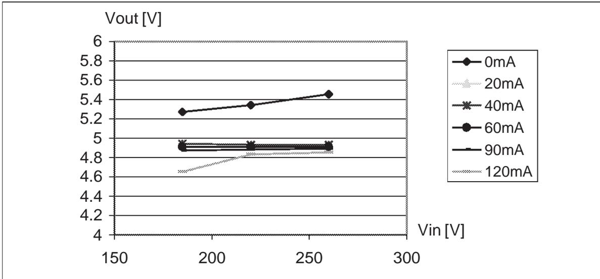
Figure 22: Buck converter with  $V_{out} = 5V$ : load regulation
