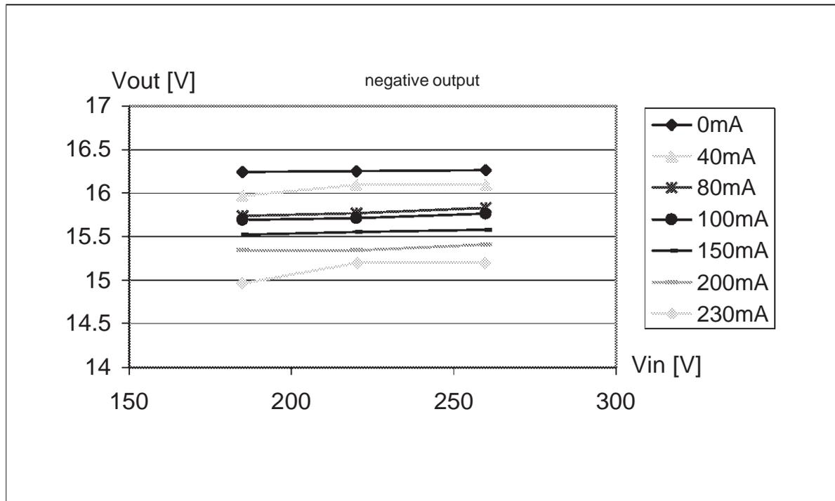
Figure 28: Buck-boost converter with  $V_{out} = -16V$ : load regulation
