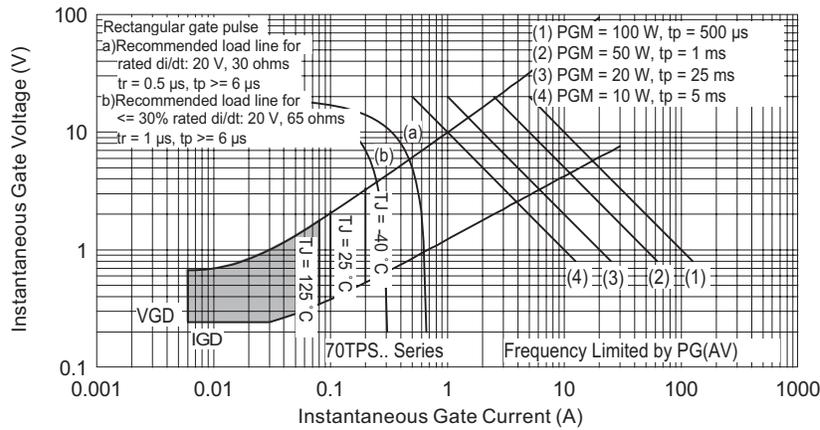
Fig. 8 - Gate Characteristics
