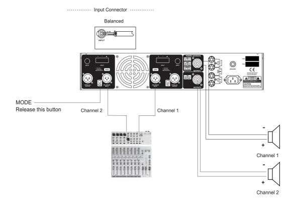
You can also operate the paralleled mode via outside wiring, so, the signal input from channel 1 or 2 will be output from both channel 1 and 2 simultaneously. The volume of channel 1 or channel 2 can be controlled separately.
