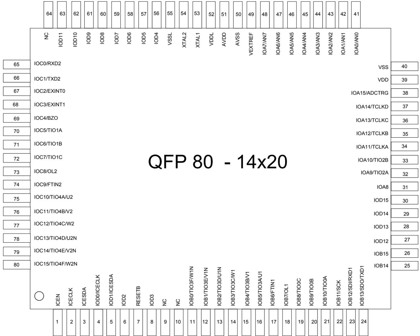
Figure 4-1 SPMC75F2413A QFP80 package
