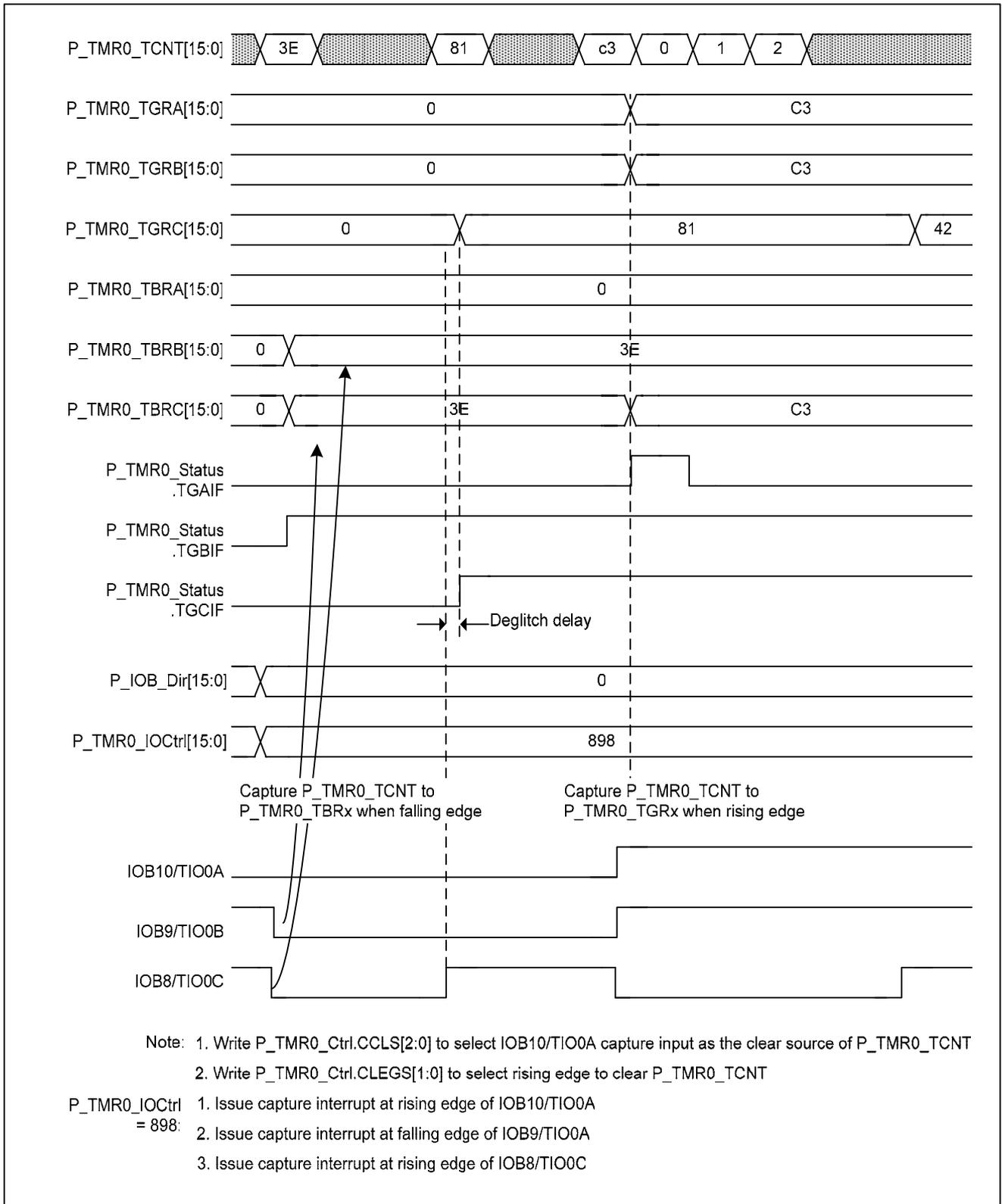
Figure 5-34 Capture input signal width and cycle
