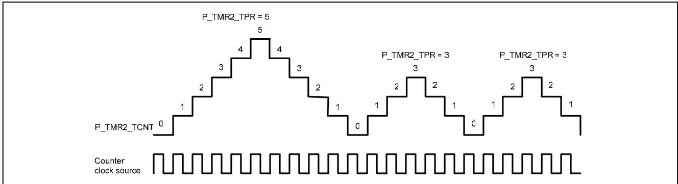
Figure 5-49 Center-Aligned mode PWM
