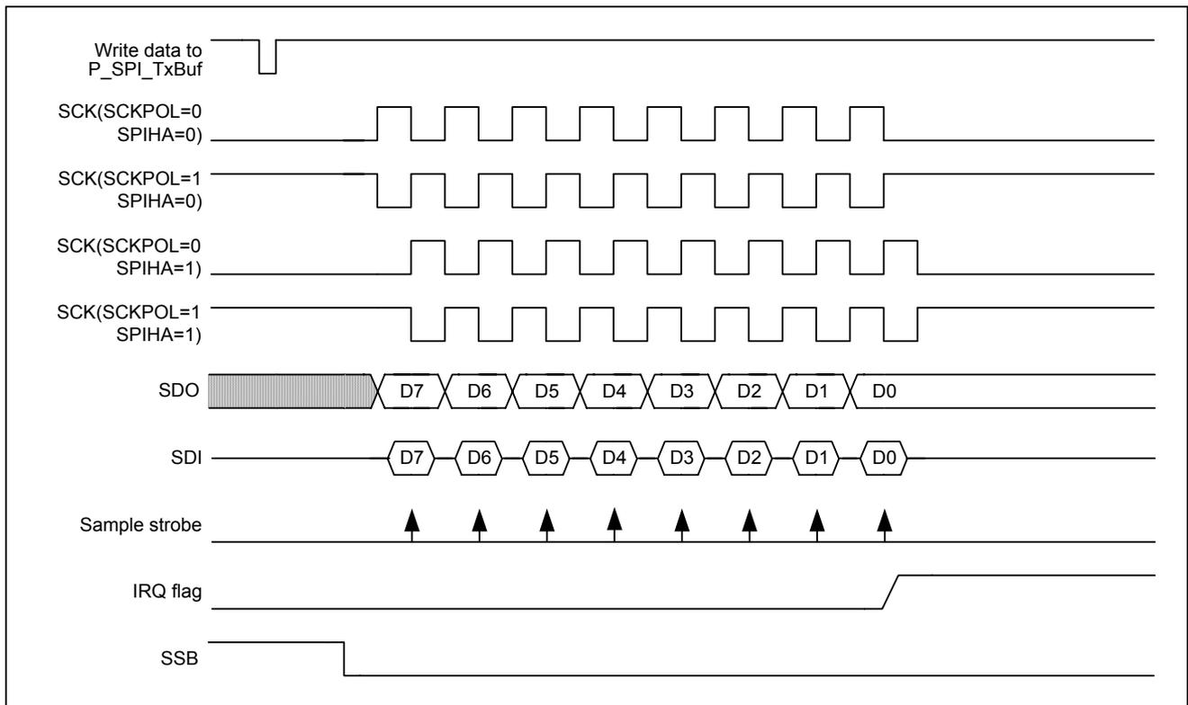
Figure 5-74 SPI mode timing, Slave Mode, SPIPHA = 0
