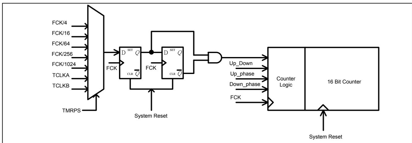
Figure 5-54 MCP timer 3 and 4 block diagram
