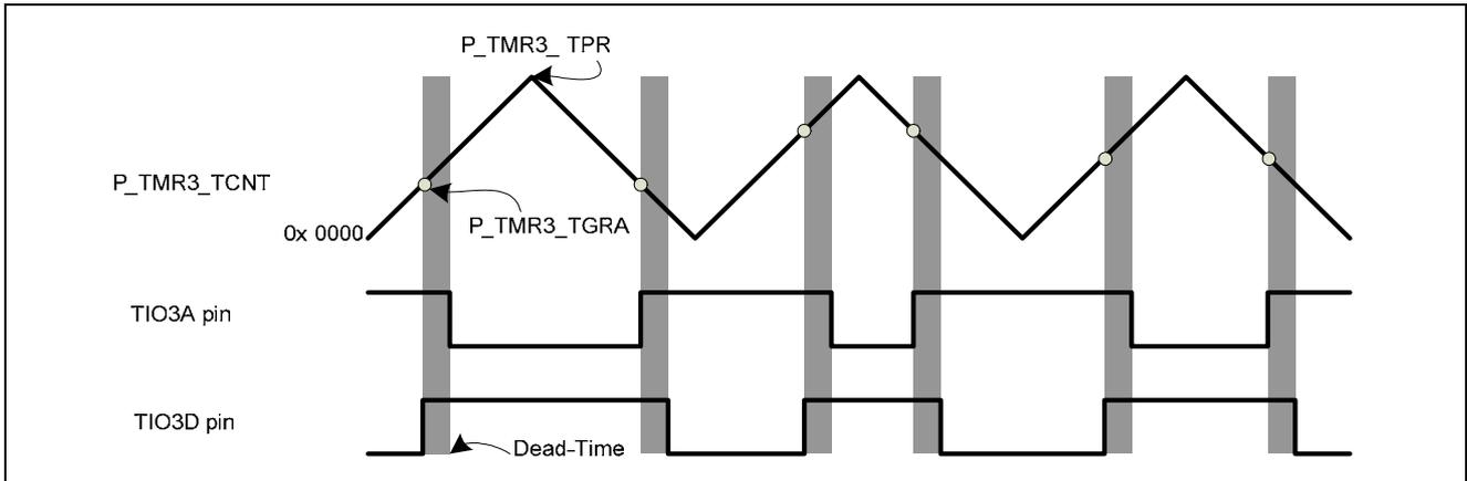
Figure 5-64 Active-low PWM mode of dead-time generation
