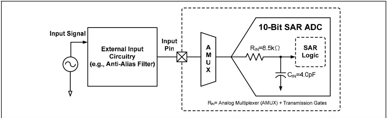
Figure 5-83 ADC equivalent circuit for SPMC75F2413A
