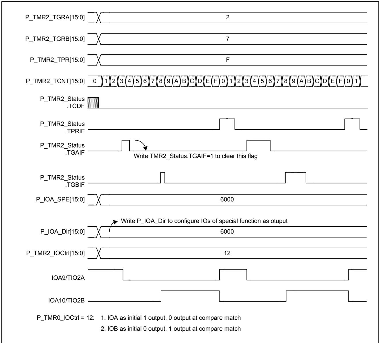
Figure 5-46 TMR2 edge aligned PWM
