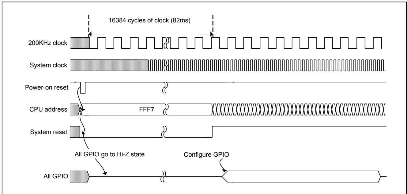
Figure 5-4 Power-up procedure
