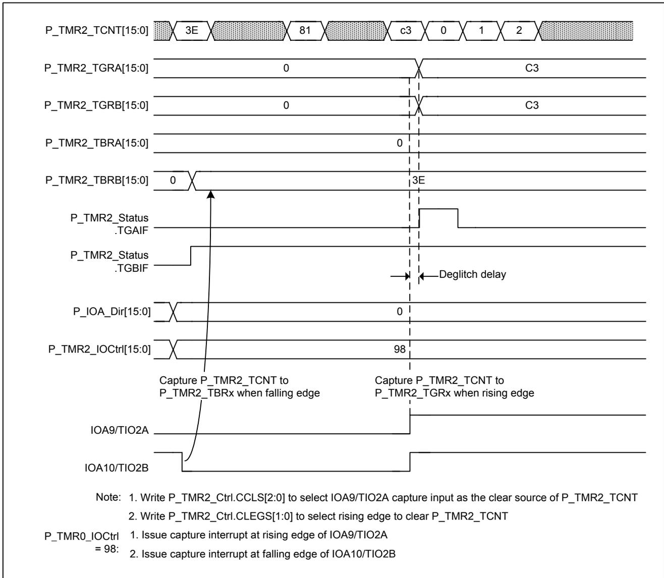
Figure 5-53 Capture input signal width and cycle
