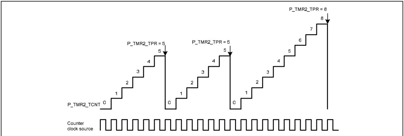
Figure 5-43 Continuous up counting example (CCLS = 111'b, CKEGS = 00'b, TMRPS = 000'b)
