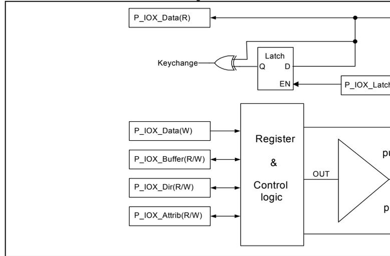
Figure 5-19 shows the structure of a typical I/O ports. The open-drain configuration can be achieved by setting the registers of direction, attribution and buffer as the following table.
