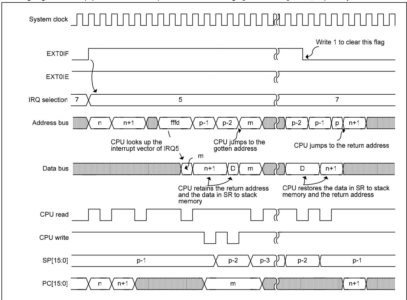
Figure 5-11 Interrupt procedure timing
