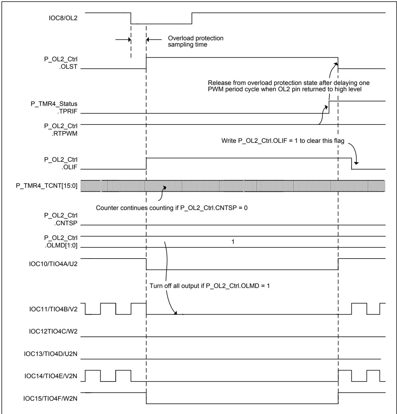
Figure 5-69 Stop all output when overload occurs
