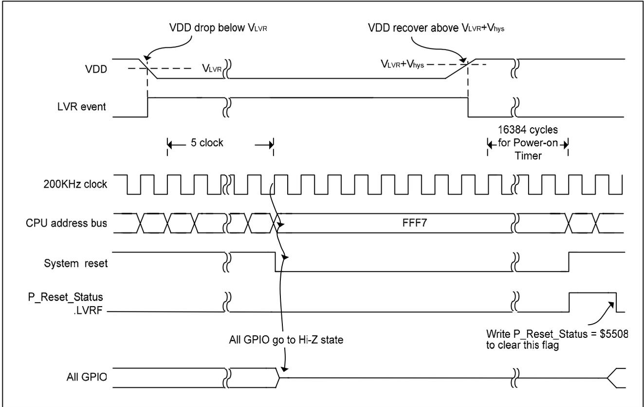
Figure 5-15 Low voltage reset timing
