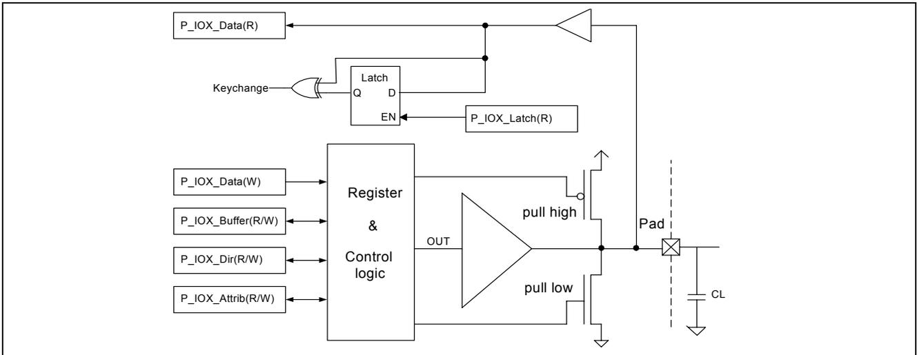
Figure 5-19 IO structure diagram
