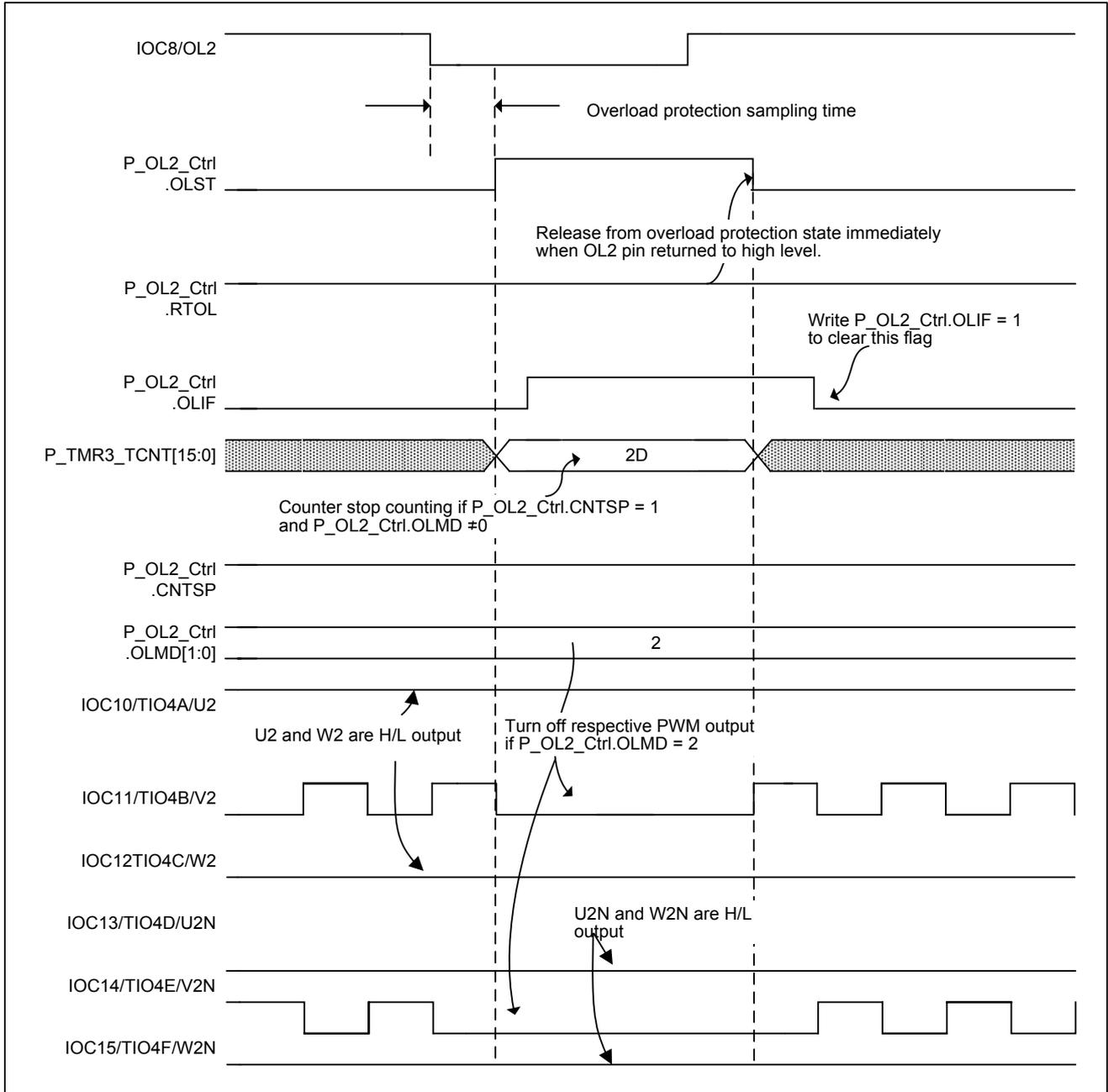
Figure 5-68 Stop PWM output only when overload occurs
