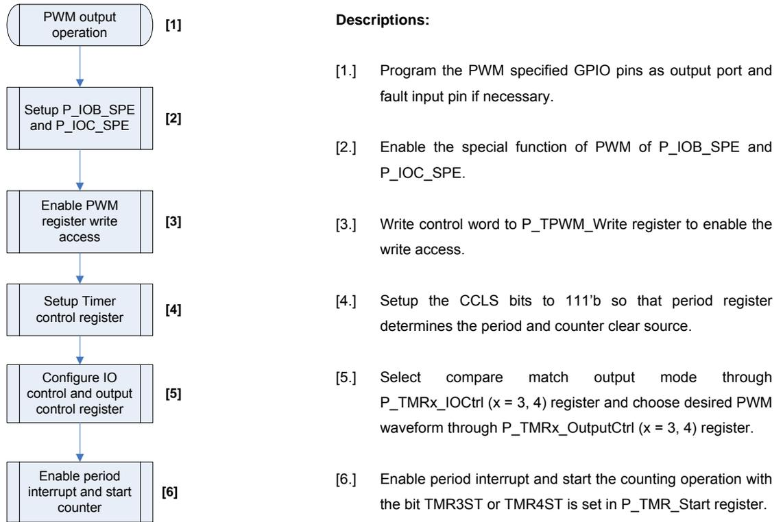
Figure 5-59 Example programming flowchart of PWM operation
