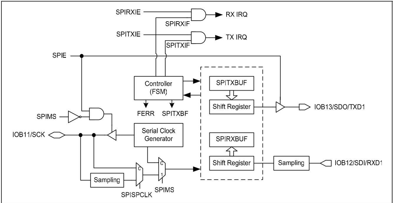
Figure 5-72 Function block diagram of SPI interface
