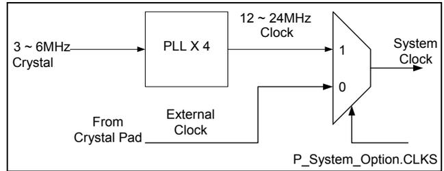
Figure 5-6 PLL and external clock block diagram
