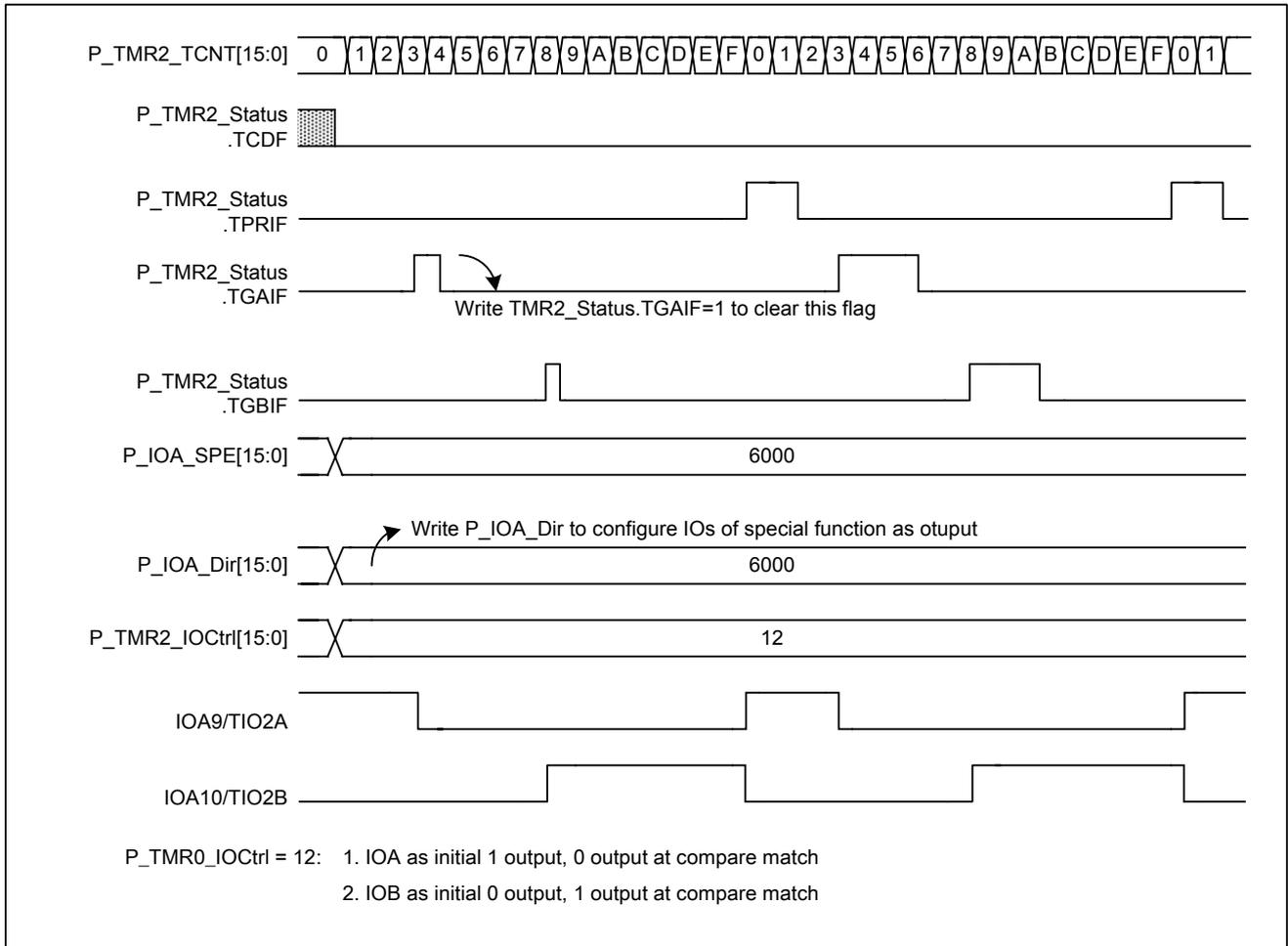
Figure 5-47 Timer mode output timing
