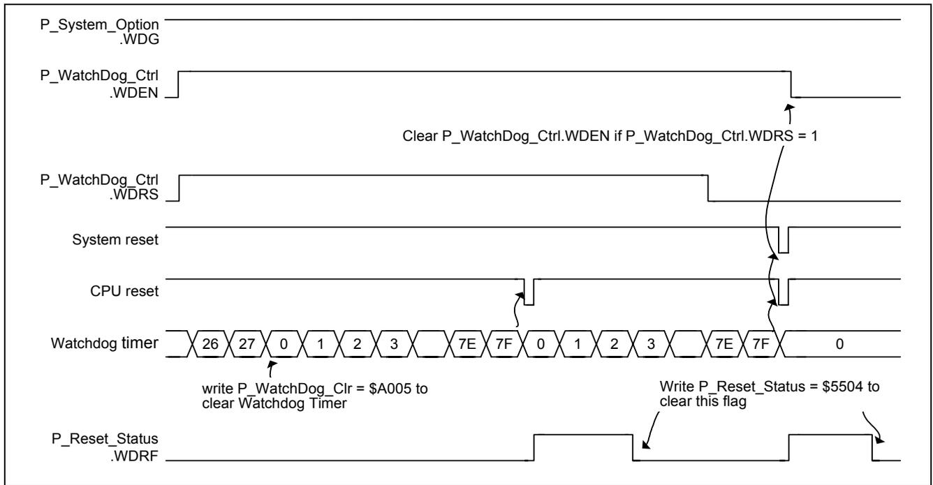
Figure 5-86 Watchdog Timing Diagram
