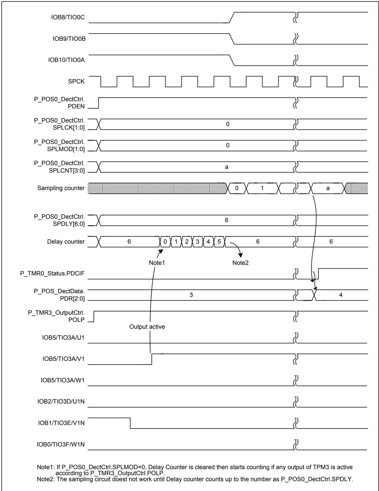
Figure 5-41 Position detection with noise filter
