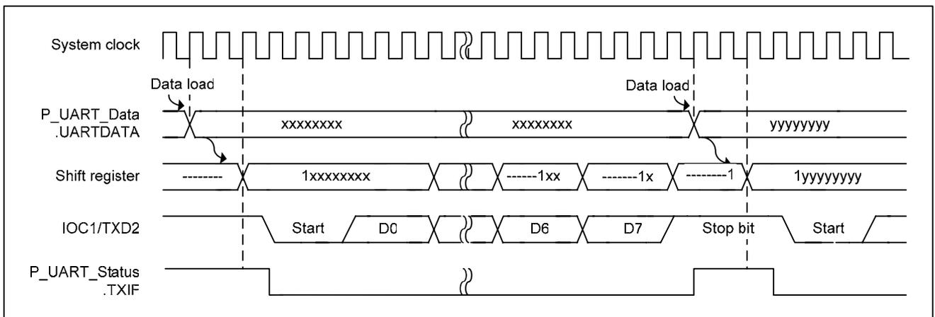
Figure 5-77 Data Transmission Timing
