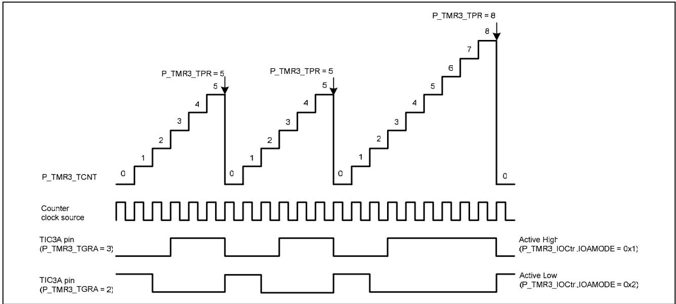
Figure 5-56 Edge-Aligned mode PWM
