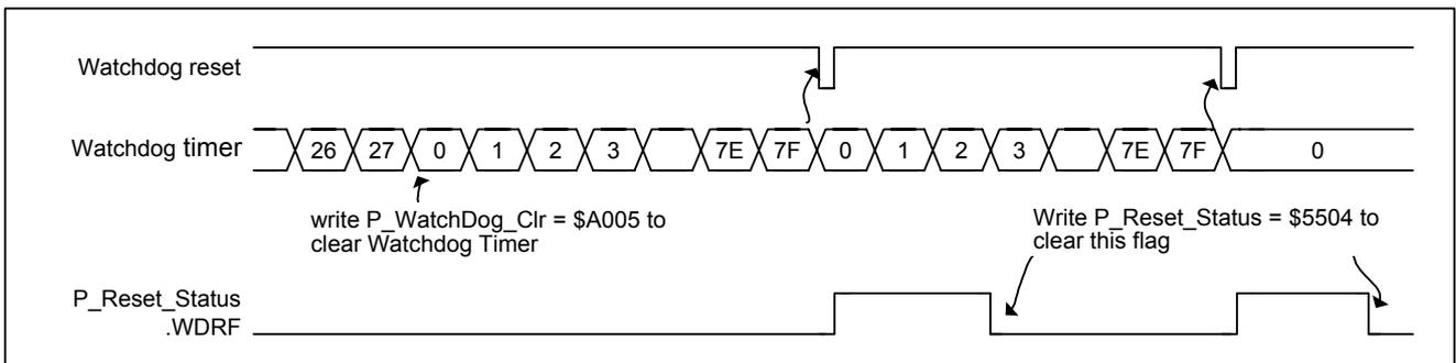
Figure 5-16 Watchdog timer reset timing
