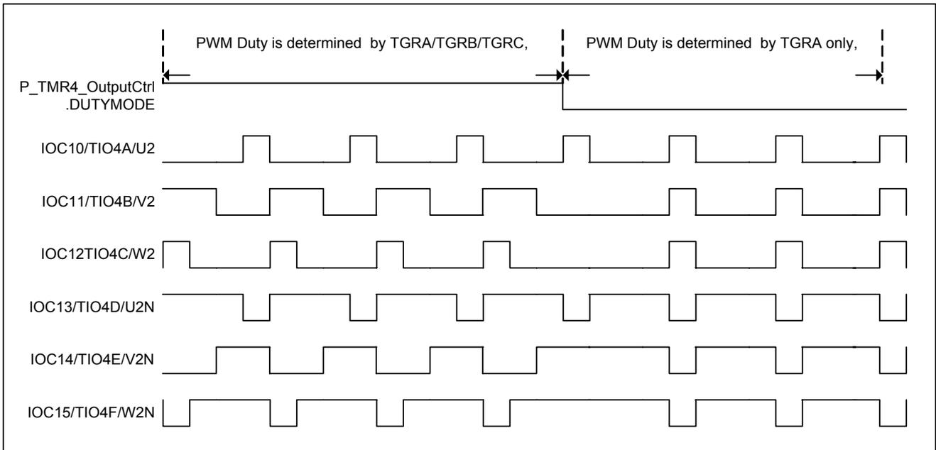
Figure 5-60 PWM output timing with different duty mode selection
