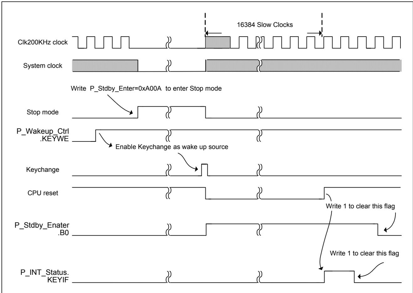
Figure 5-10 Standby mode timing
