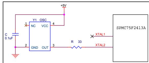
Figure 5-7 The external clock from oscillator connection
