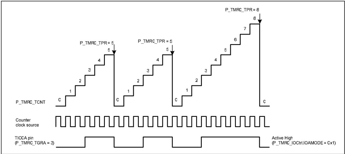
Figure 5-25 Edge-Aligned mode PWM
