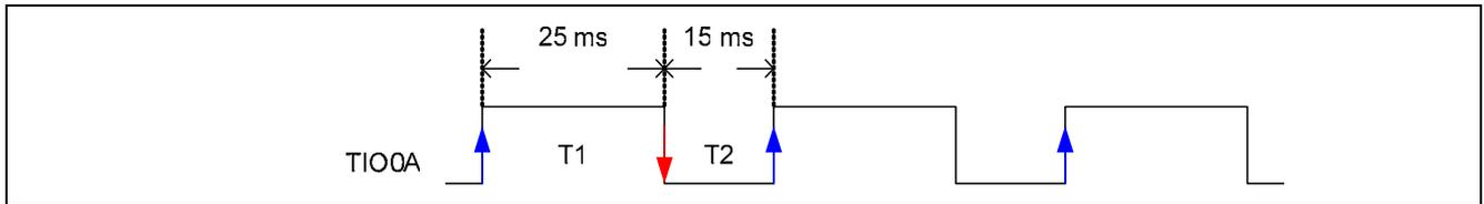
Figure 5-32 input capture signal connected to TIO0A
