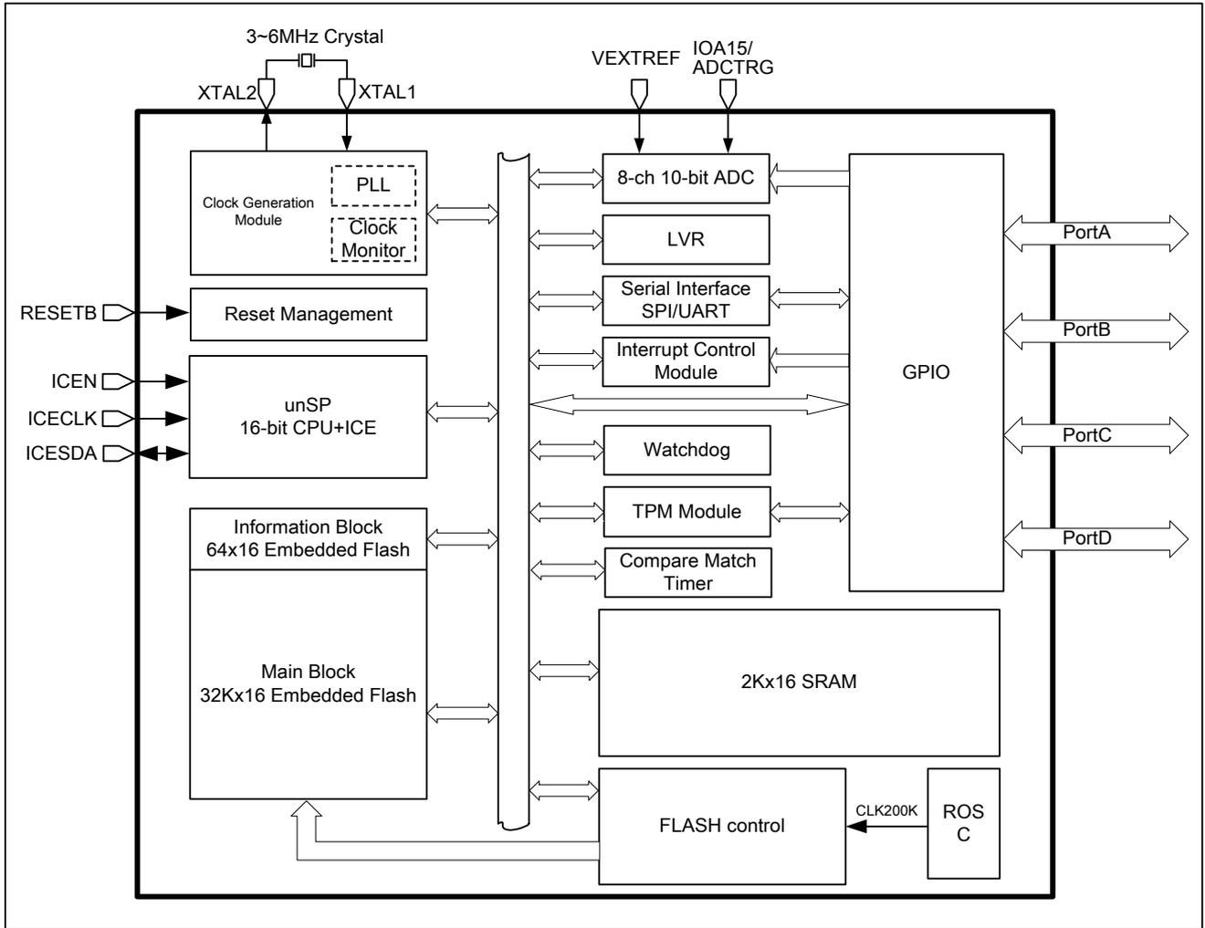
Figure 3-1 SPMC75F2413A function block diagram
