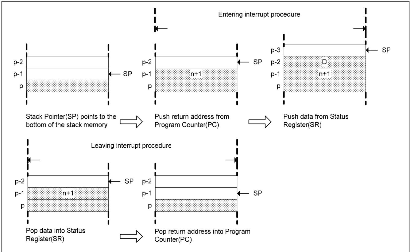
Figure 5-12 Stack memory operation with interrupt procedure
