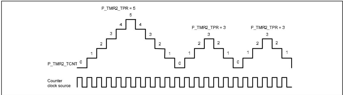
Figure 5-48 Continuous up/down counting example (CCLS = 111'b, CKEGS = 00'b, TMRPS = 000'b)
