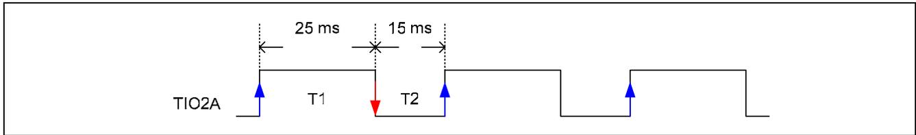
Figure 5-51 input capture signal connected to TIO2A
