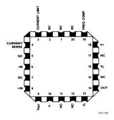
Connection Diagram 10-Lead Can (Top View)
