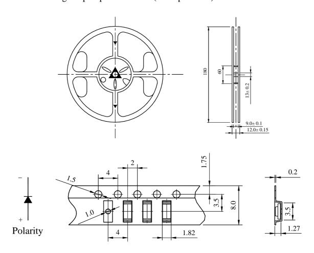
Reel Lead Min.60mm No LEDs
