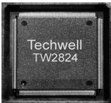
TW2824 208-pin PQFP package
