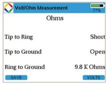
The Volt/Ohm mode identifies the presence of an open, short, or resistance on a line
