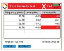
The NIT helps users locate isolation issues in coax cable to identify which legs contain faults that could allow ingress into the coax network
