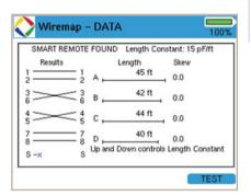
Twisted Pair Wire Map helps technicians find impairments and incorrect wiring in phone and Ethernet cables
