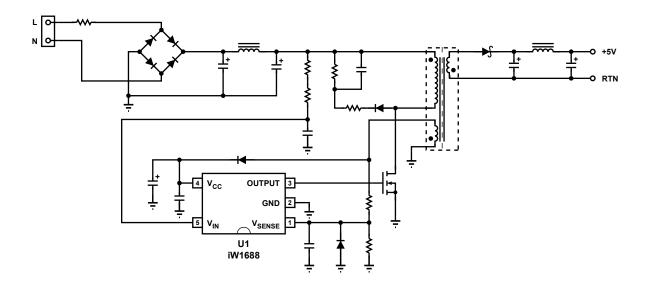
Figure 2.0.1 iW1688 Typical Application Circuit
