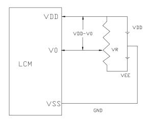
Vdd-V0: LCD Driving Voltage
