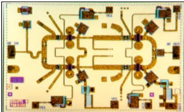
The TriQuint TGA1071-EPU is a two stage PA MMIC design using TriQuint's proven 0.25 um Power pHEMT process to support a variety of millimeter wave applications including point-to-point digital radio and point-to-multipoint systems.
