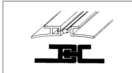
Loc-Trac® provides an effective closure that is ideal for use where the assembly will be subjected to random flexing.
