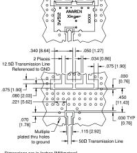
Dimensions are in Inches [Millimeters] 3W512 Rev A Mounting Footprint
