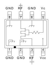
1.  $V_{CC} = +3 V_{DC} @ 50 \mu A max.$
