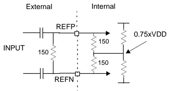
**Figure 7. Reference Clock Termination**
