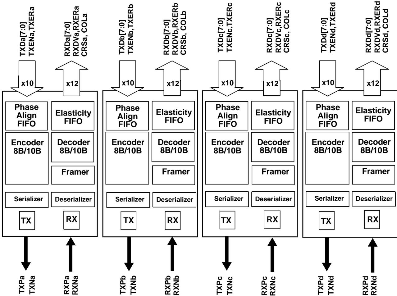
Figure 2. CYP32G0401DX Transceiver Logic Block Diagram
