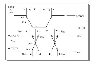
Note: See Switching Wave Forms for the definition of the switching terms. Supplies must be by-passed with .01  $\mu F$  Capacitors. Unused inputs must be tied to Ground
