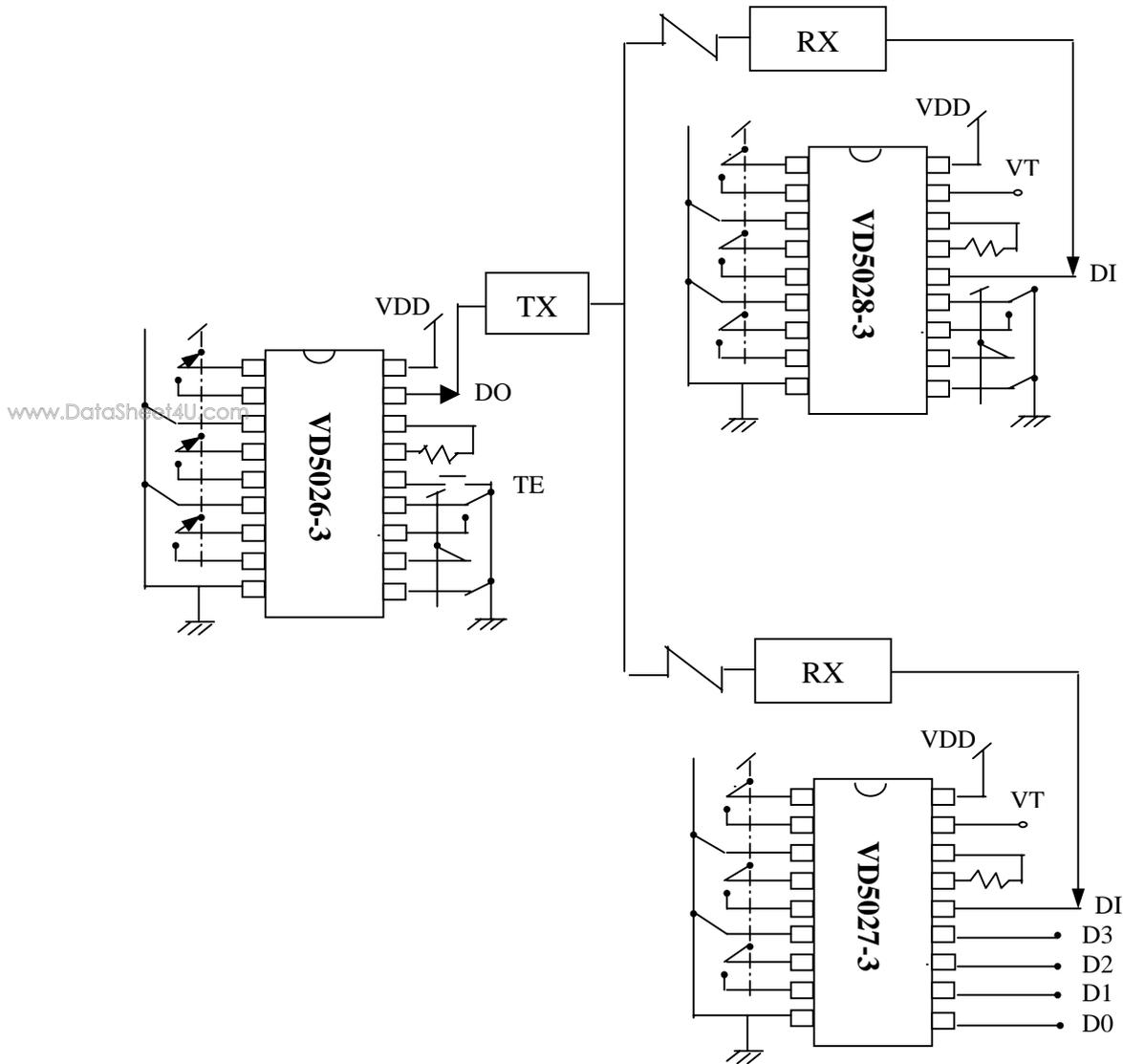
The IC substrate should be connected to  $V_{DD}$ . 芯片襯底請接 $V_{DD}$ .
