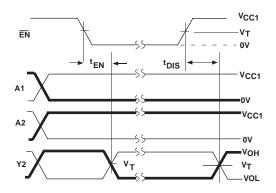
Figure 3. Y2 Enable and Disable Times
