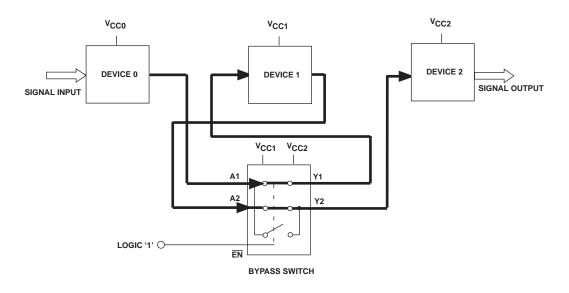
Figure 4. Bypass Switch in Normal Mode
