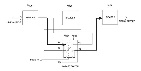
Figure 5. Bypass Switch in Bypass Mode
