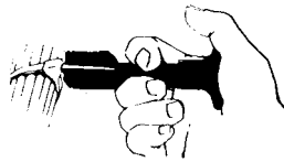
1. With tie in hand—squeeze to tension. Insert cable tie into cable tie head, then squeeze tool to proper tension.
