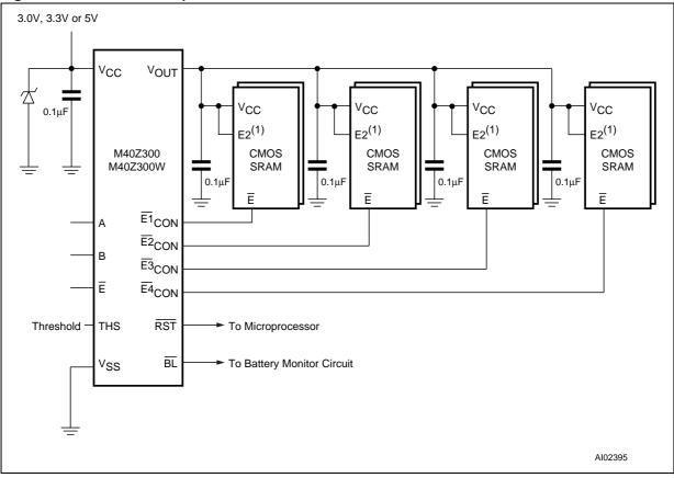
Note: 1. If the second chip enable pin (E2) is unused, it should be tied to  $V_{\mbox{OUT}}.$
