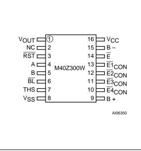
Note: For M40Z300W, B- must be connected to the negative battery terminal only (not to Pin 8, V<sub>SS</sub>).
