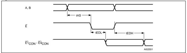
Note: During system design, compliance with the SRAM timing parameters must comprehend the propagation delay between  $\overline{E1}_{CON}$  -  $\overline{E4}_{CON}$ .
