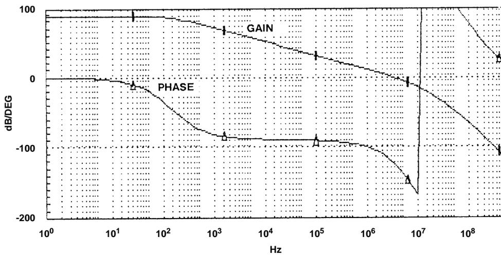
FIGURE 1. GAIN/PHASE RESPONSE vs FREQUENCY
