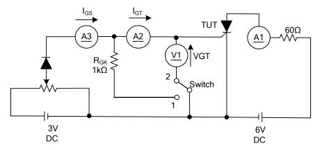
Switch 1: I<sub>GT</sub> Measurement Switch 2: V<sub>GT</sub> Measurement
