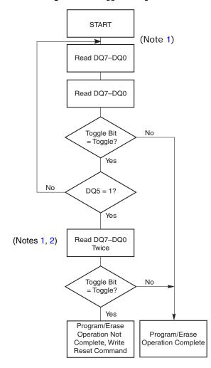
Figure 11.2 Toggle Bit Algorithm
