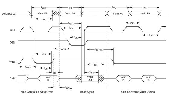
Figure 17.7 Back to Back Read/Write Cycle Timing
