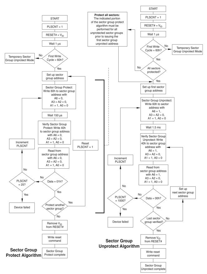
Figure 7.2 In-System Sector Group Protect/Unprotect Algorithms
