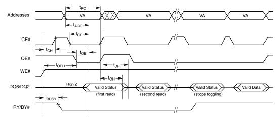
Figure 17.9 Toggle Bit Timings (During Embedded Algorithms)
