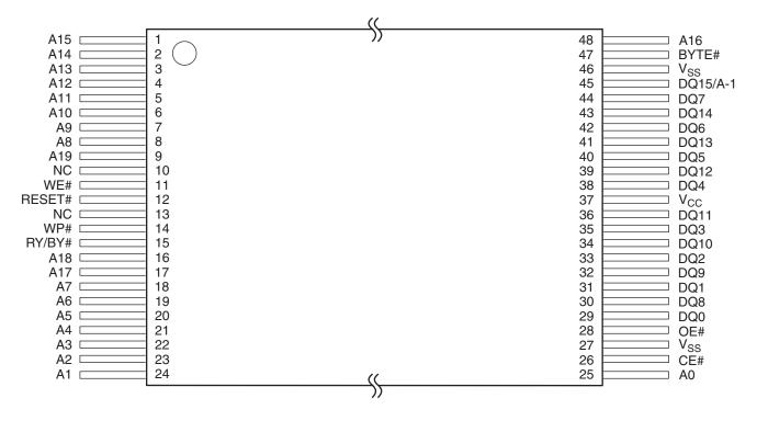
Figure 3.1 48-pin Standard TSOP (TS048)
