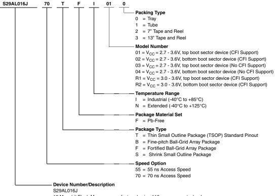
16 Megabit Flash Memory manufactured using 110 nm process technology 3.0 Volt-only Read, Program, and Erase
