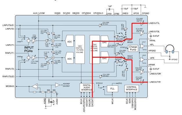
Figure 64 Stereo DAC to Line Output 1 Device Internal Signal Path
