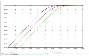
ADC Digital High Pass Filter Ripple.
