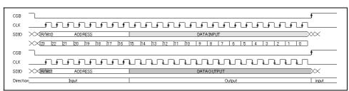
Figure 47 3-Wire Serial Control Timing
