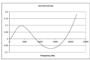
Figure 58 De-Emhpasis Digital Filter Response (44.1kHz)
