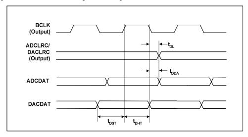
Figure 5 Digital Audio Data Timing - Master Mode
