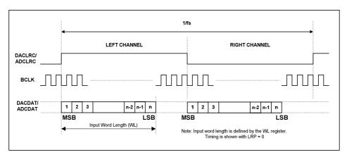
Figure 32 Left Justified Audio Interface (assuming n-bit word length)
