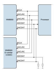
Figure 31 TDM with Processor as Master
