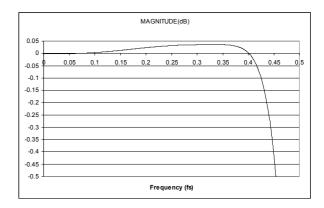
Figure 55 DAC Digital Filter Ripple (Sloping Stopband Mode)
