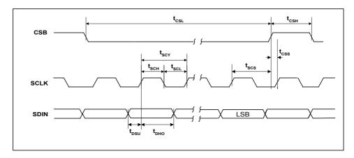
Figure 8 Control Interface Timing – 3-Wire Serial Control Mode
