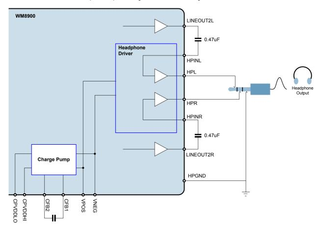
Figure 20 Ultra-Low Power Ground-Referenced Headphone Output
