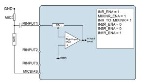
Figure 12 Single-ended Microphone Configurations
