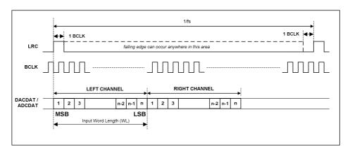
Figure 38 DSP/PCM Mode Audio Interface (mode B, AIF\_LRCLKINV =0, Slave)
