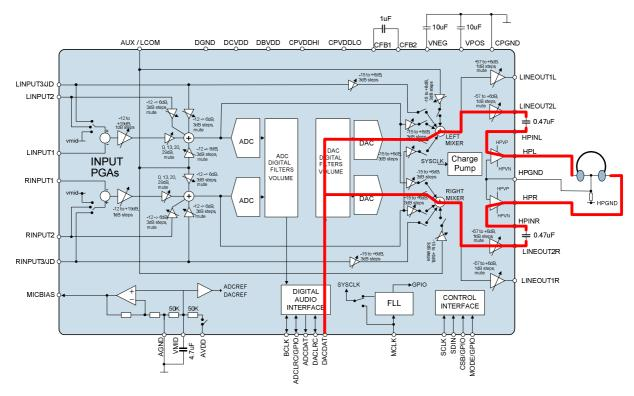
Figure 63 Stereo DAC to Headphone Device Internal Signal Path
