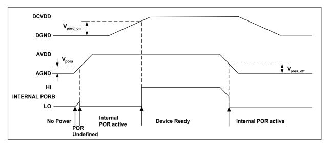
Figure 10 Typical Power up Sequence where AVDD is Powered before DCVDD
