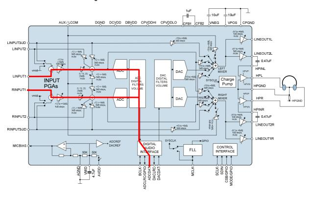
Figure 65 L/RINPUT1 to ADC Internal Signal Path - Recommended Power up Sequence and Device Register Settings
