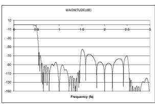
Figure 54 DAC Digital Filter Frequency Response (Sloping Stopband Mode)
