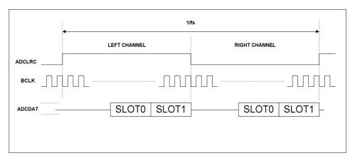
Figure 40 TDM in Right-Justified Mode
