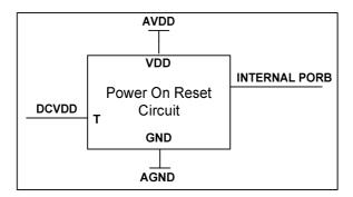
Figure 9 Internal Power on Reset Circuit Schematic
