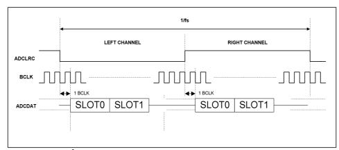
Figure 41 TDM in I<sup>2</sup>S Mode
