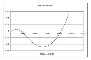
Figure 60 De-Emhpasis Digital Filter Response (48kHz)
