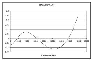
Figure 56 De-Emhpasis Digital Filter Response (32kHz)
