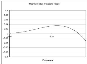
Figure 50 ADC Digital Filter Frequency Response
