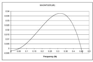
Figure 52 DAC Digital Filter Frequency Response (Normal Mode)
