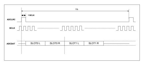
Figure 42 TDM in DSP/PCM Mode A
