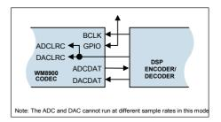
Figure 27 Master Mode with ADCLRC as GPIO
