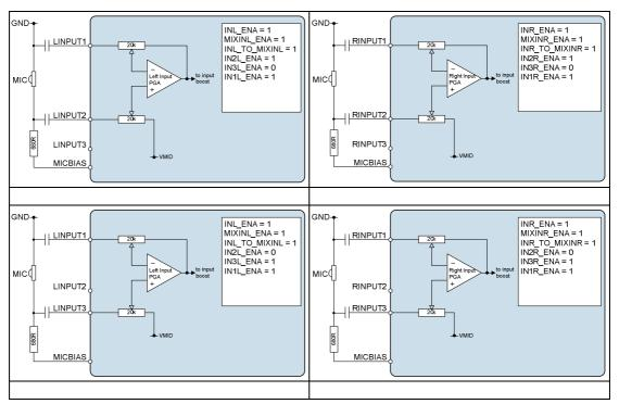
Figure 13 Differential Microphone Input Configurations
