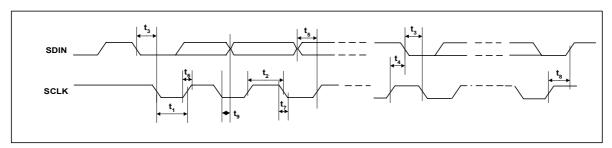
Figure 7 Control Interface Timing – 2-Wire Serial Control Mode
