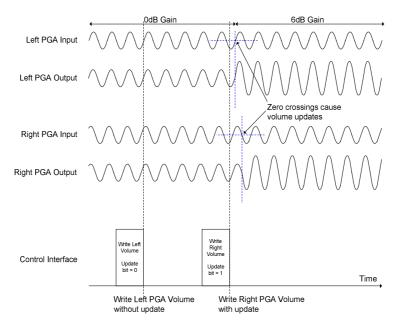
Figure 23 Volume Update Using Zero Cross Detection
