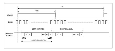
Figure 35 DSP/PCM Mode Audio Interface (mode A, AIF\_LRCLKINV=0, Master)
