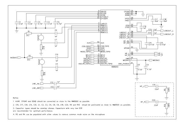
Figure 1 External Component Connectivity
