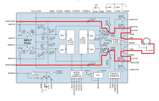
Figure 66 LR Input 3 to Headphone Bypass Path
