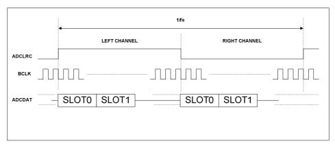
Figure 39 TDM in Left-Justified Mode
