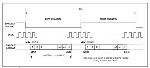
Figure 34 I<sup>2</sup>S Justified Audio Interface (assuming n-bit word length)
