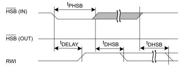
$\overline{\text{HSB}}$  pin is driven high to V<sub>CCQ</sub> only by Internal 100 KΩ resistor, HSB driver is disabled SRAM is disabled as long as  $\overline{\text{HSB}}$  (IN) is driven LOW.
