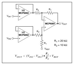
**FIGURE 4-6:** Instrumentation Amplifier with Unity-Gain Buffer Inputs.
