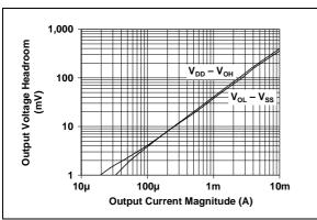
**FIGURE 2-14:** Output Voltage Headroom vs. Output Current Magnitude.
