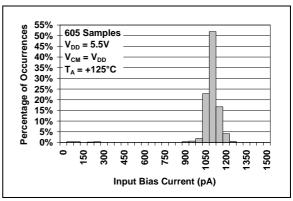
FIGURE 2-6: Input Bias Current at +125°C.
