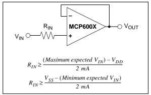
**FIGURE 4-2:** Input Current Limiting Resistor  $(R_{IN})$ .
