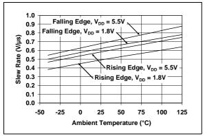
**FIGURE 2-13:** Slew Rate vs. Ambient Temperature.
