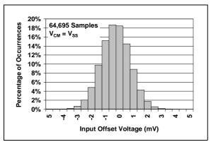
FIGURE 2-1: Input Offset Voltage.
