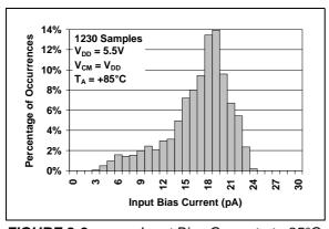
FIGURE 2-3: Input Bias Current at +85°C.
