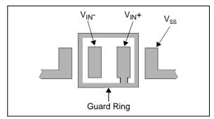
**FIGURE 4-5:** Example Guard Ring Layout for Inverting Gain.
