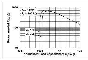
**FIGURE 4-4:** Recommended R<sub>ISO</sub> values for Capacitive Loads.
