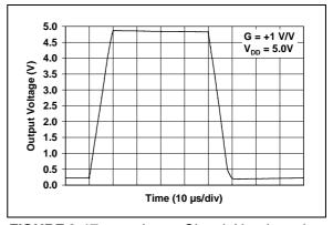
**FIGURE 2-17:** Large-Signal, Non-Inverting Pulse Response.
