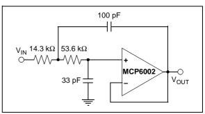
FIGURE 4-7: Active Second-Order Low- Pass Filter.
