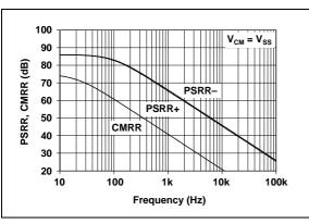
**FIGURE 2-2:** PSRR, CMRR vs. Frequency.
