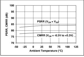
**FIGURE 2-4:** CMRR, PSRR vs. Ambient Temperature.
