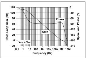
FIGURE 2-5: Open-Loop Gain, Phase vs. Frequency.
