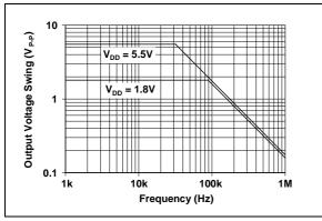
**FIGURE 2-15:** Output Voltage Swing vs. Frequency.
