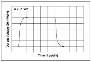
**FIGURE 2-16:** Small-Signal, Non-Inverting Pulse Response.
