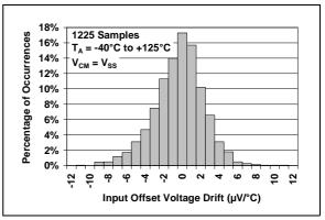
FIGURE 2-10: Input Offset Voltage Drift.
