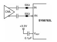
Figure 2c. AC-Coupling to CML Driver
