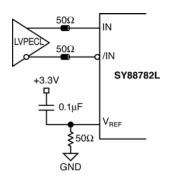
Figure 2a. DC-Coupling to LVPECL Driver
