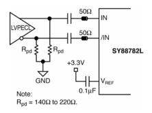
Figure 2b. AC-Coupling to LVPECL Driver
