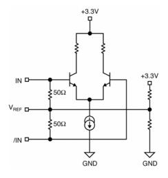
Figure 1a. Simplified Input Stage
