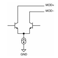
Figure 1b. Simplified Output Stage
