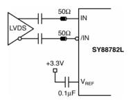
Figure 2d. AC-Coupling to LVDS Driver
