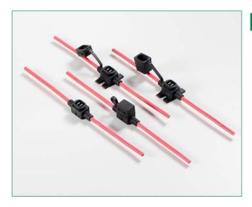
This product is an In-line fuse holder for use with either standard or Low Profile JCASE™ fuses, 20A - 60A. It offers size and weight savings compared to MAXI™ fuseholders, and has an optional protective cover for splash resistance. Standard product will have two 102mm red wire leads. Wire length and insulation color can be customized upon request. Tinned wires also available upon request. All customizations have minimum order requirements. Contact Littelfuse sales representative for details.
