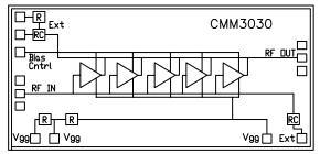
controlled to maintain correct drain current and thus drain voltage. The typical gate voltage needed to do this is 0.0V. Typically the gate is protected with Silicon diodes to limit the applied voltage. Also, make sure to sequence the applied voltage to ensure negative gate bias is available before applying the positive drain supply.
