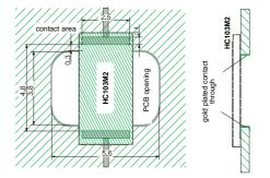
To allow full access of the air, the humidity sensor should be positioned over an opening in the printed circuit board (PCB).
