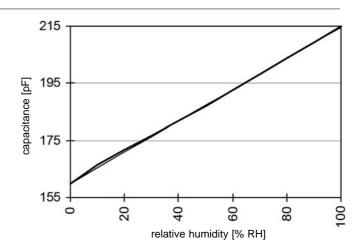
For high accuracy requirements, the sensitivity is determined by the following polynomial:
