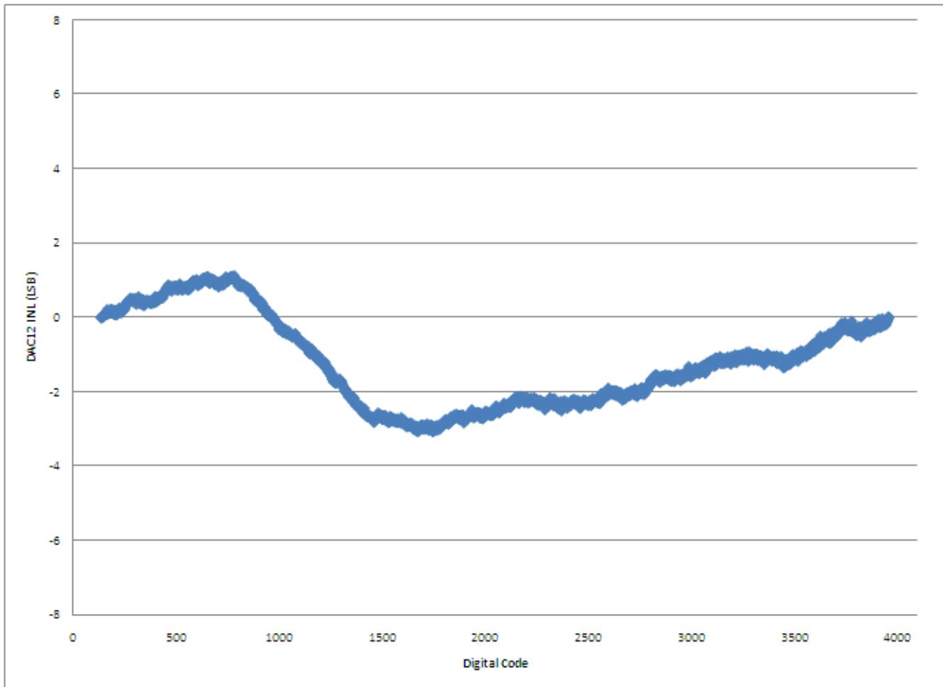
Figure 15. Typical INL error vs. digital code
