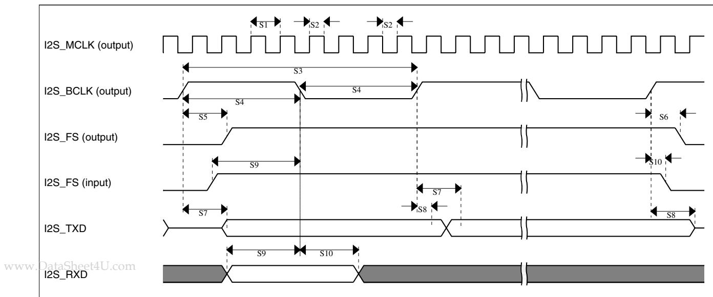
**Figure 24. I<sup>2</sup>S timing — master mode**
