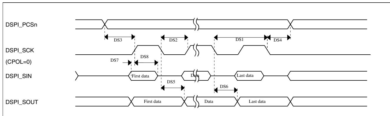
**Figure 19. DSPI classic SPI timing — master mode****Table 37. Slave mode DSPI timing (low-speed mode)**
