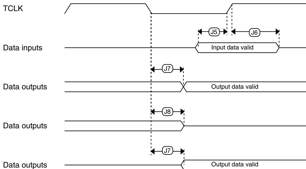
**Figure 6. Boundary scan (JTAG) timing**
