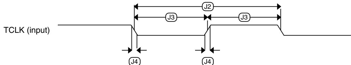
**Figure 5. Test clock input timing**
