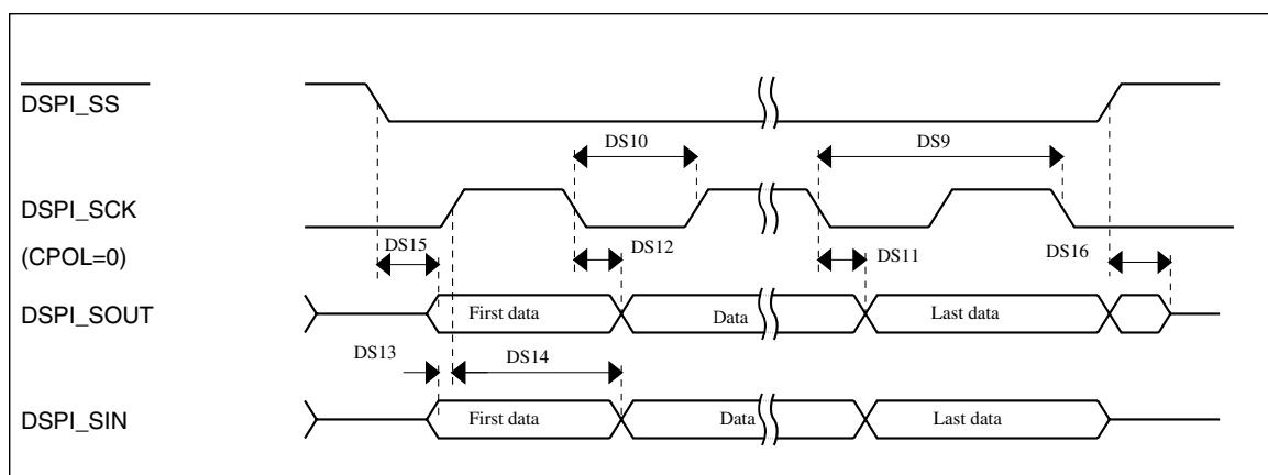
**Figure 22. DSPI classic SPI timing — slave mode**
