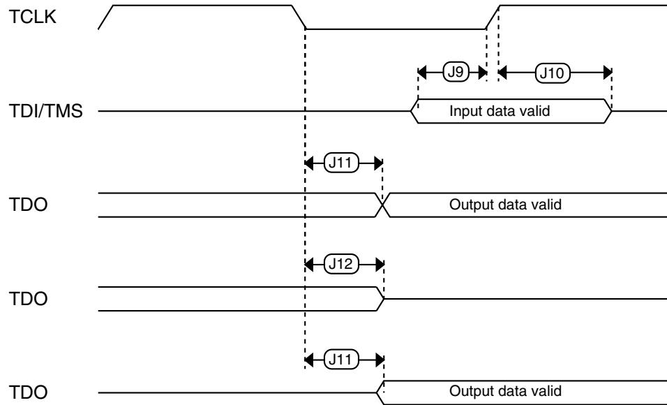
**Figure 7. Test Access Port timing**
