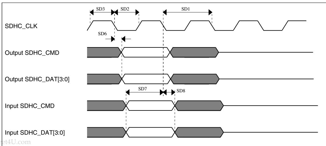
**Figure 23. SDHC timing**
