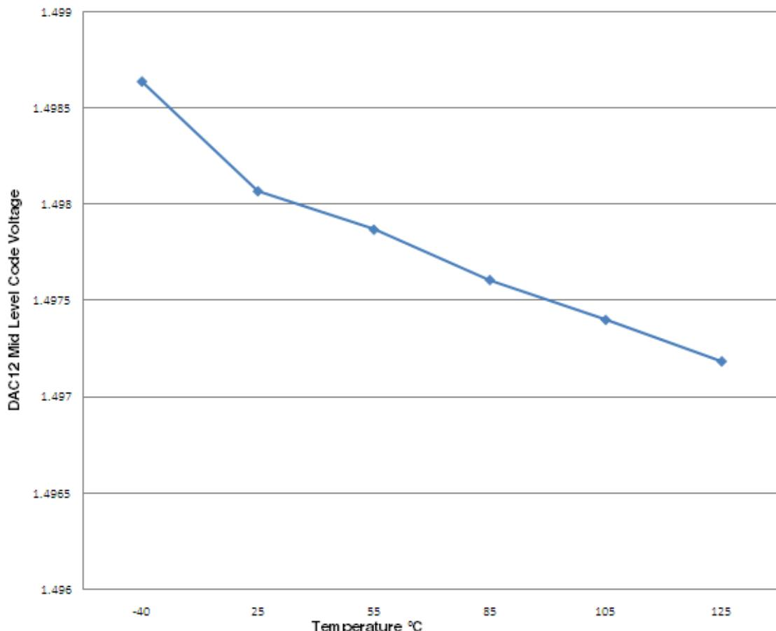
**Figure 16. Offset at half scale vs. temperature**
