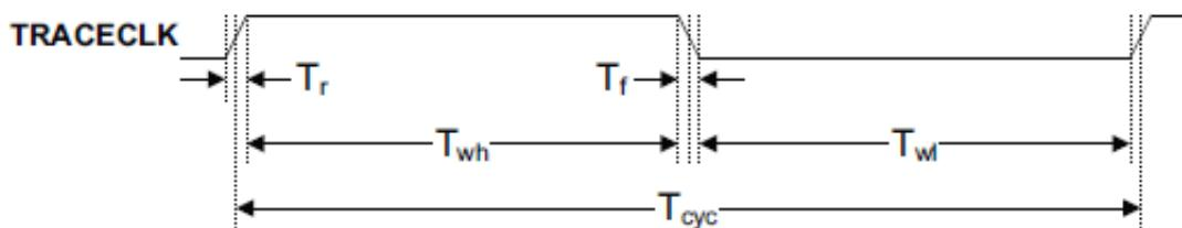
**Figure 3. TRACE\_CLKOUT specifications**
