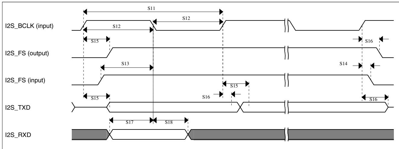
**Figure 25. I<sup>2</sup>S timing — slave modes**
