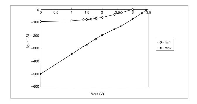
**DC Characteristics** (Ta = 0 to +70°C,  $V_{CC}$ ,  $V_{CC}Q = 3.3 \text{ V} \pm 0.3 \text{ V}$ ,  $V_{SS}$ ,  $V_{SS}Q = 0 \text{ V}$ ) (HM5259165B)
