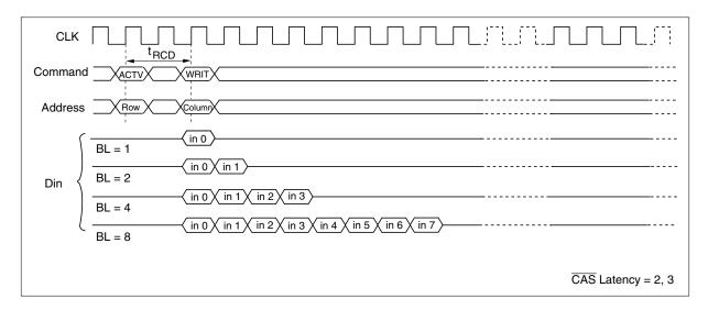
**2. Single write:** A single write operation is enabled by setting OPCODE (A9, A8) to (1, 0). In a single write operation, data is only written to the column address and the bank select address (BA0/BA1) specified by the write command set cycle without regard to the burst length setting. (The latency of data input is 0 clock).
