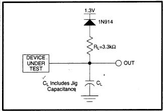
Figure 16. Transient Equivalent Testing Load Circuit
