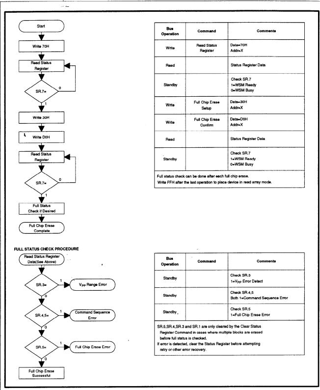
Figure 6. Automated Full Chip Erase Flowchart
