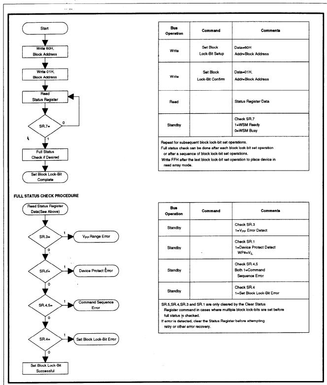
Figure 12. Set Block Lock-Bit Flowchart
