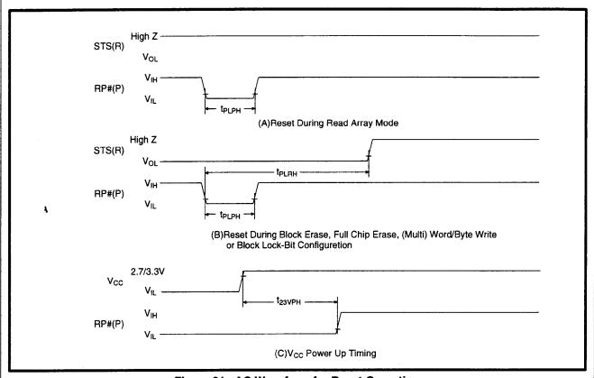
Figure 21. AC Waveform for Reset Operation
