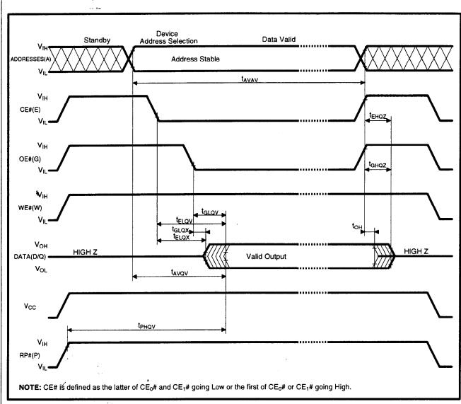
Figure 17. AC Waveform for Read Operations
