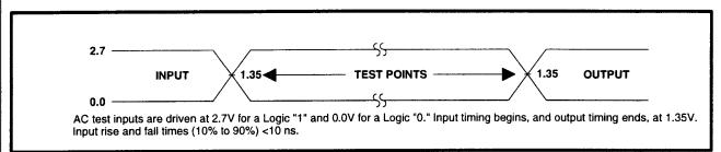
Figure 14. Transient Input/Output Reference Waveform for V<sub>CC</sub>=2.7V-3.6V
