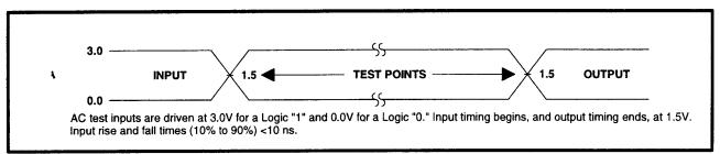
Figure 15. Transient Input/Output Reference Waveform for V<sub>CC</sub>=3.3V±0.3V
