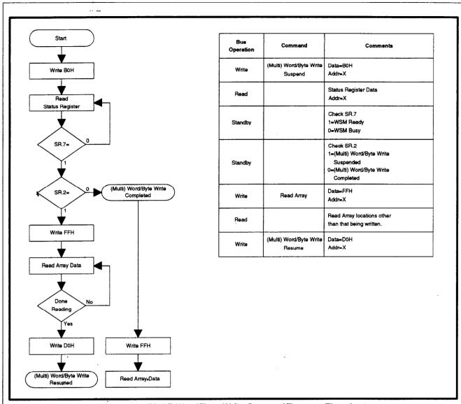
Figure 11. (Multi) Word/Byte Write Suspend/Resume Flowchart
