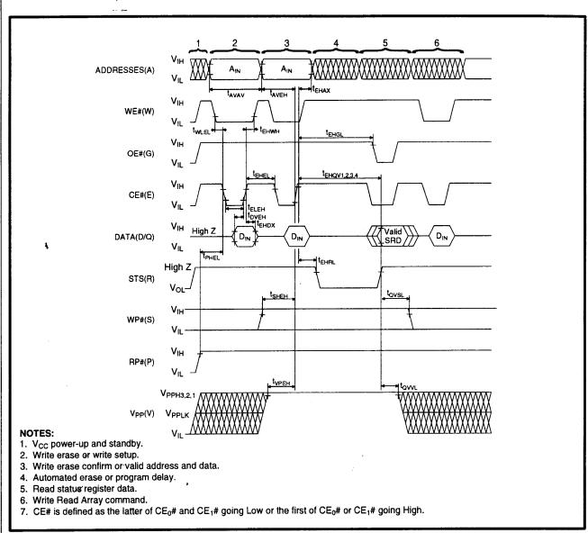
Figure 20. AC Waveform for CE#-Controlled Write Operations
