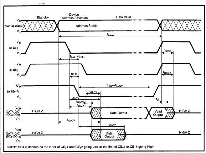
Figure 18. BYTE# Timing Waveforms
