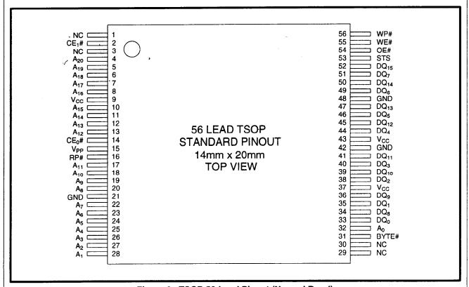
Figure 2. TSOP 56-Lead Pinout (Normal Bend)
