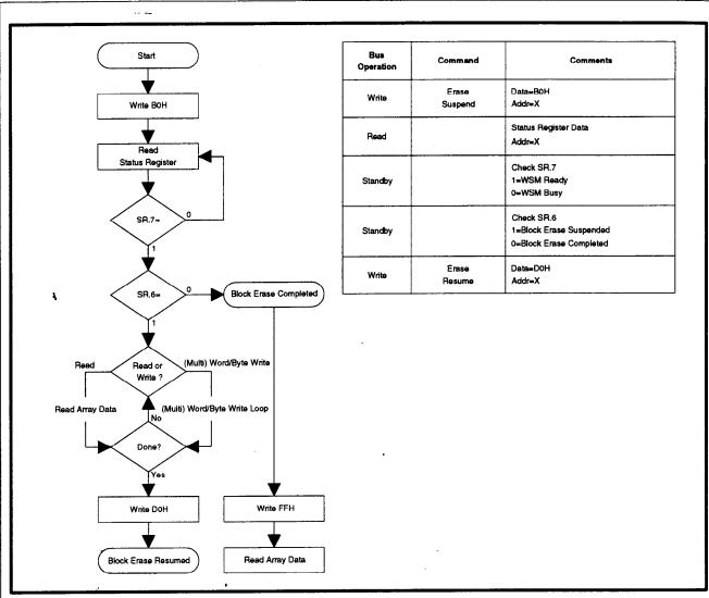
Figure 10. Block Erase Suspend/Resume Flowchart
