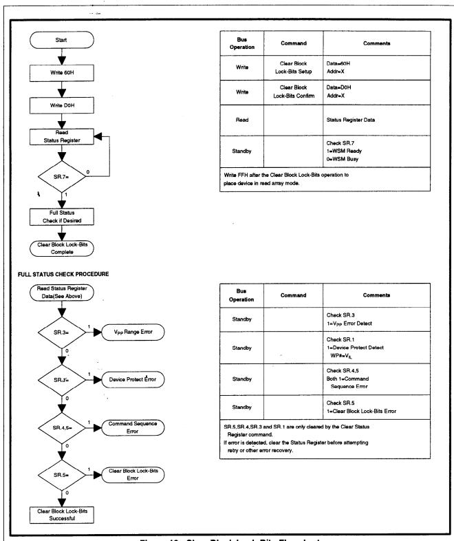
Figure 13. Clear Block Lock-Bits Flowchart
