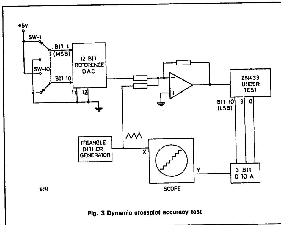
Switches SW-1 to SW-10 are set to the appropriate digital code to select the point on the characteristic to be displayed. For example, code 10000 00000 would select half full-scale, i.e. the major transition.
