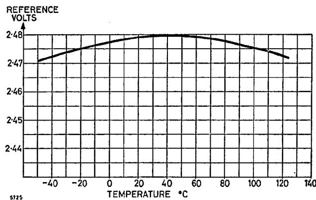
Fig. 6 Typical reference voltage v temperature (all types)
