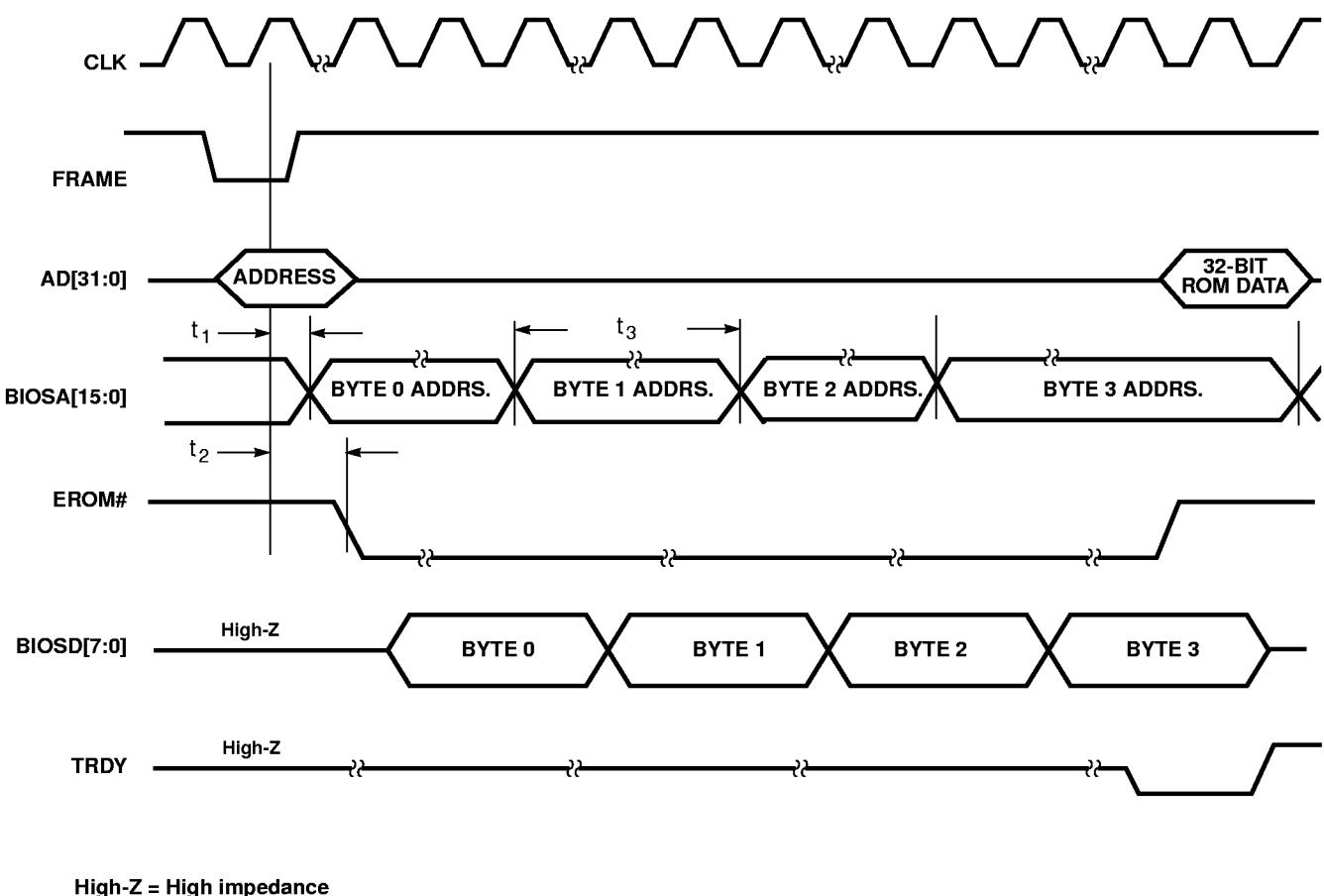
**Figure 11-2. EROM#, BIOSA[15:0] Timing (PCI Bus)**
