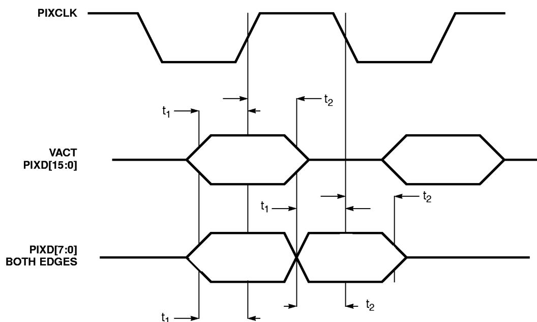
**Figure 11-6. V-Port™ – PIXCLK Timing**
