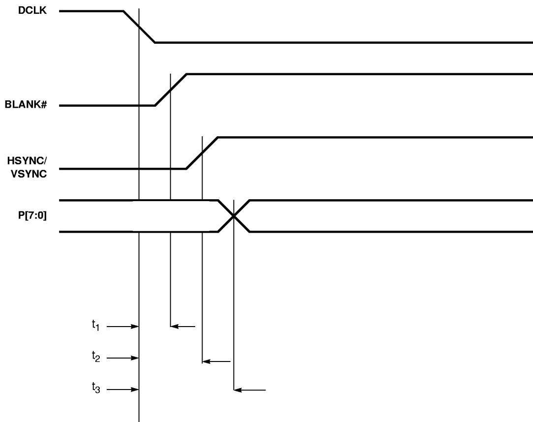
**Figure 11-5. Feature Bus Timing – Output (Internal DCLK)**
