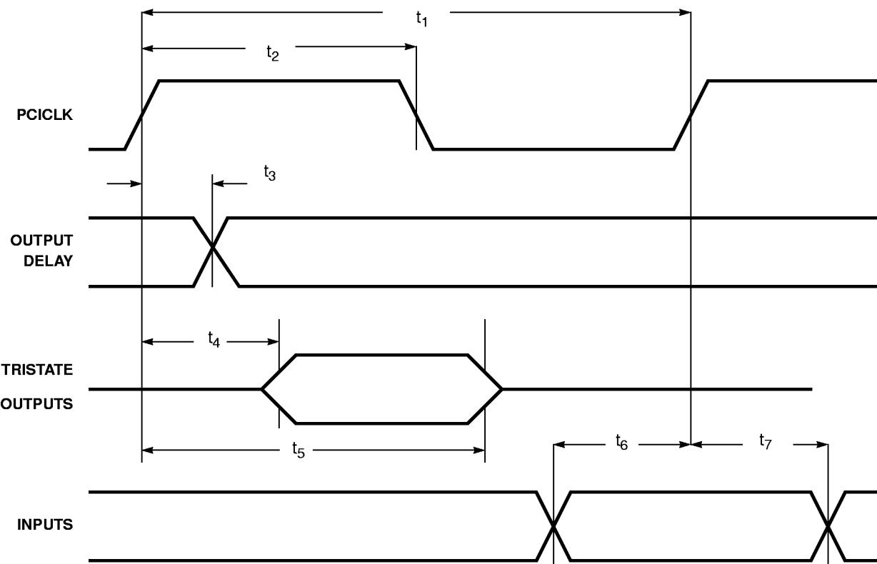
**Figure 11-1. PCI Bus Timing**
