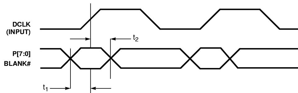
**Figure 11-4. P-Bus as Inputs (External DCLK)**
