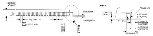
All dimension in mm (inches). Notation is  $\frac{MAX}{MIN}$  or typical.
